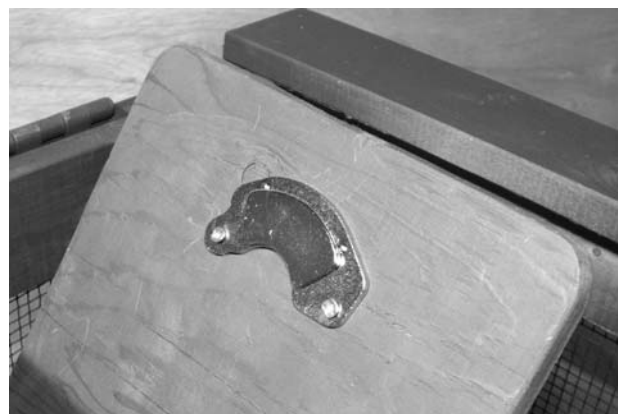
Figure 11-19 A hard disk drive magnet holds the can in place
