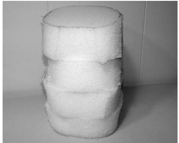
Figure 6-18 Foam disks glued and ready to cut
