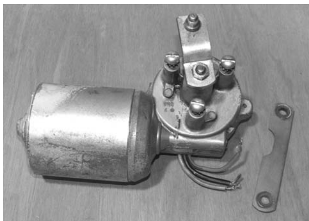
Figure 10-23 The bare wiper motor cleaned and tested
