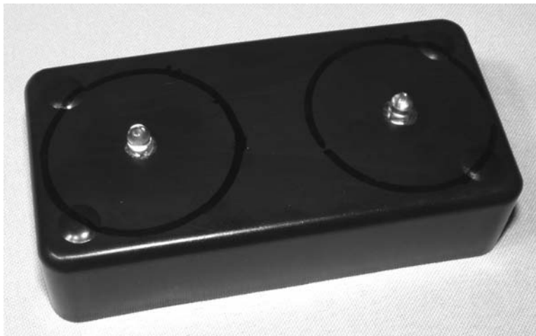
Figure 5-3 Mounting the LEDs in the plastic box
