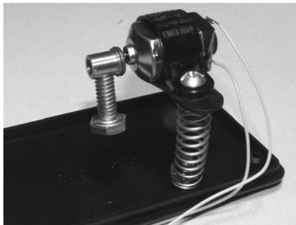
Figure 4-29 A spring mounted motor for serious noise
