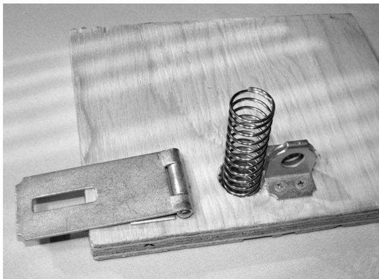
Figure 3-23 The hinge is now spring loaded
