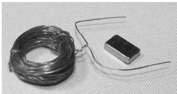
Figure 5-20 Finished coil and a tiny NIB magnet
