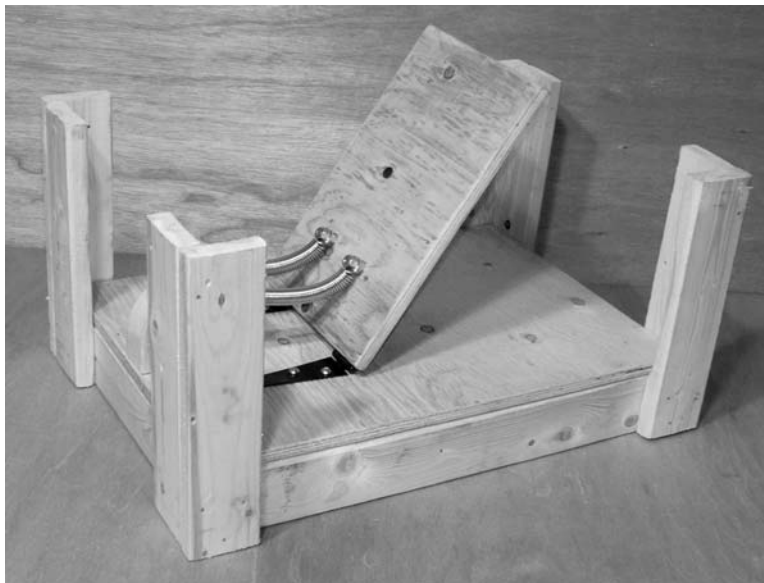
Figure 11-7 Cage base and side supports installed
