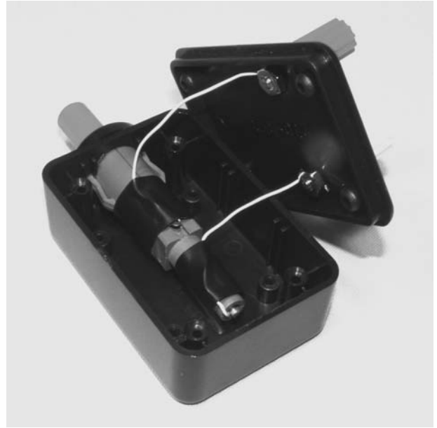
Figure 7-3 Installing the igniter in a case
