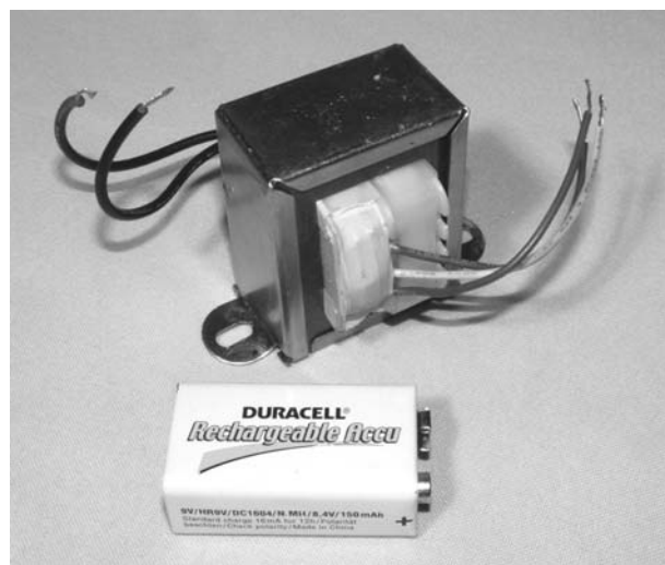
Figure 7-5 An AC transformer and a battery
