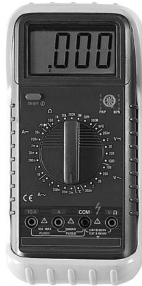
Figure 1-4 A basic multi-meter for electronics work
