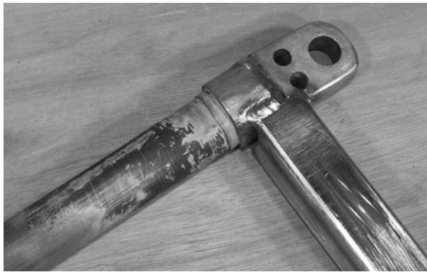
Figure 5-72 Welding the brake support arms
