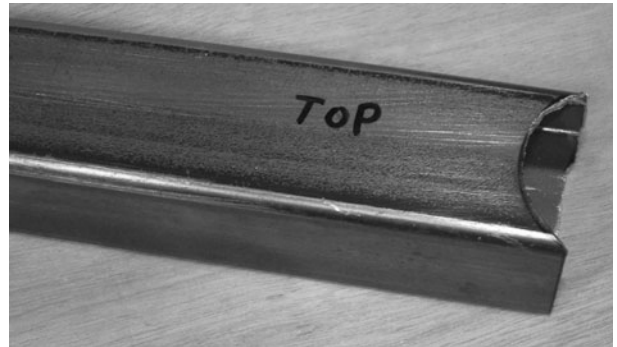
Figure 5-47 Cutting the fish mouth for the head tubes
