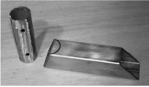
Figure 6-85 Trace out the area to be cut
