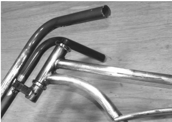
Figure 3-14 New forks installed
