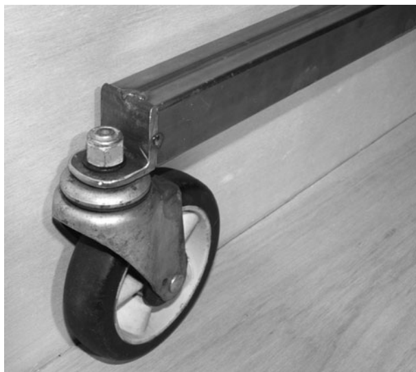
Figure 8-18 Check caster alignment before finalizing the welds
