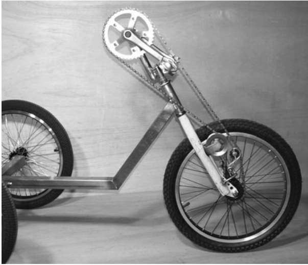
Figure 9-66 Chain installed and drive system complete
