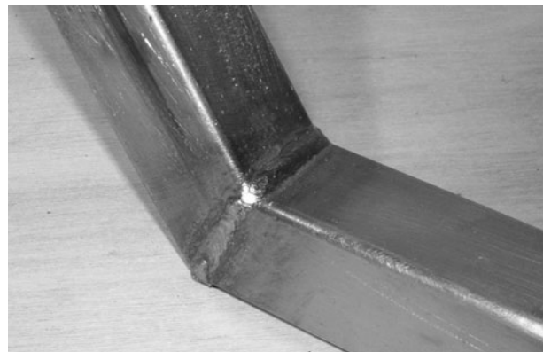
Figure 9-19 A good solid weld is needed here
