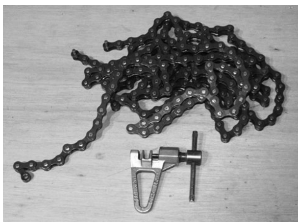
Figure 6-125 Joining two bicycle chains
