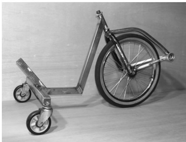
Figure 8-28 Tack welded T-bar ready for adjustment
