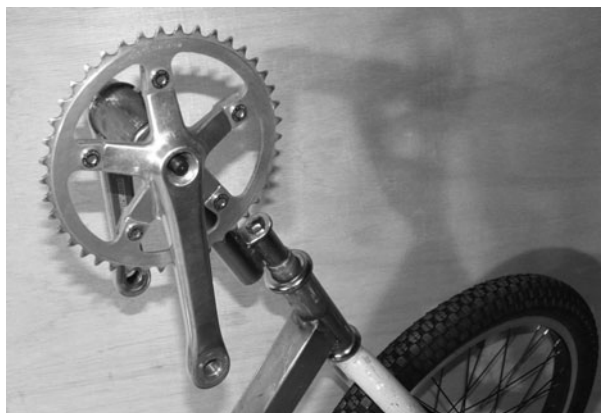
Figure 9-50 Crank arms are installed in the same direction
