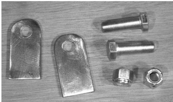
Figure 5-75 Steering control arms and bolts
