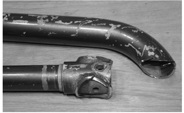
Figure 5-7 Cutting the fork legs from the stem
