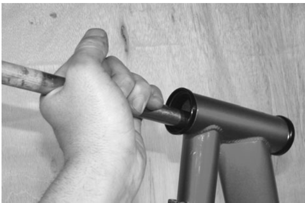
Figure 1-22 Removing the head tube cups
