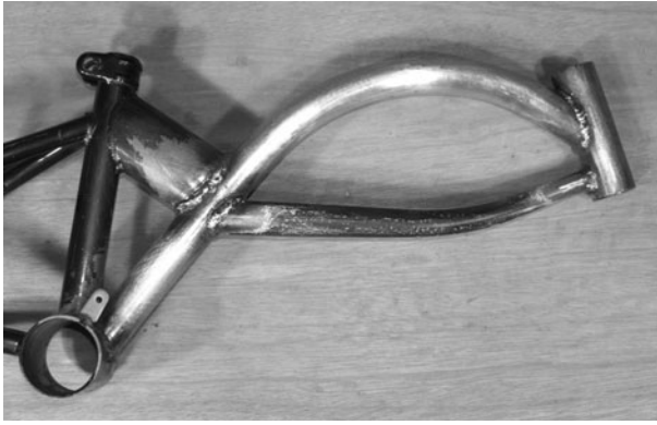
Figure 4-12 Completing the frame welds
