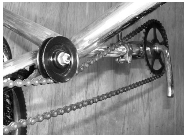
Figure 7-20 Chain idler pulley installed
