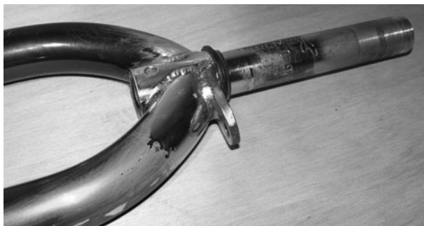
Figure 6-109 Make this weld solid
