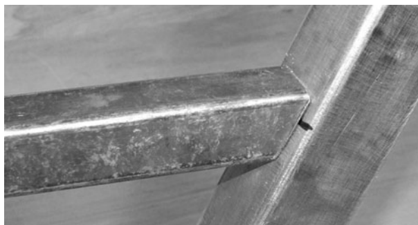
Figure 13-35 Keeping the top tube parallel to the rear boom
