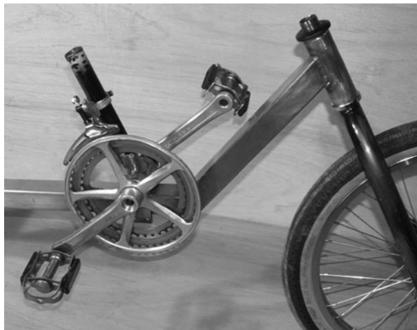
Figure 6-100 Bottom bracket installed into the frame
