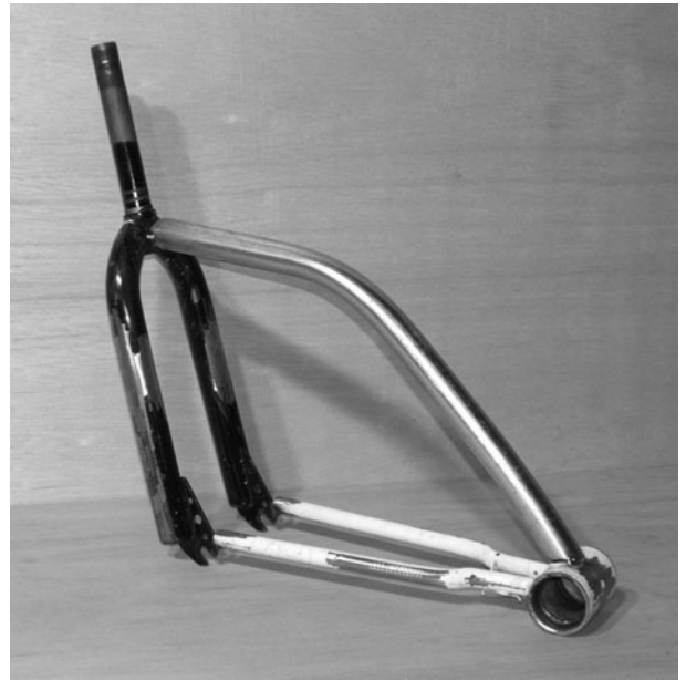
Figure 8-10 The front end tack welded together
