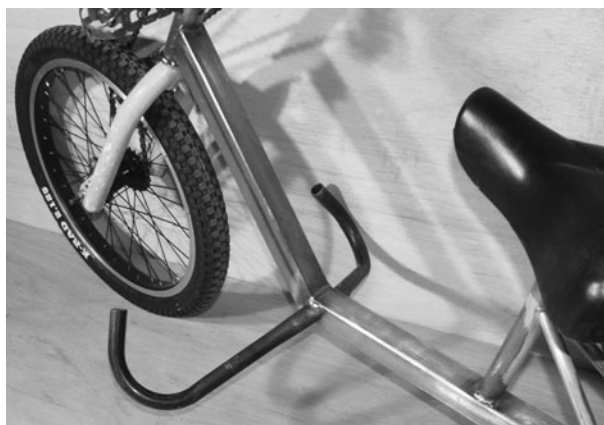
Figure 9-77 Leg mount tubes tack welded in place
