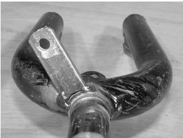
Figure 7-22 Steering control arm welded to the fork
