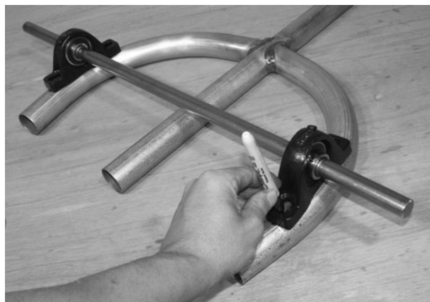
Figure 2-40 A good bearing alignment trick
