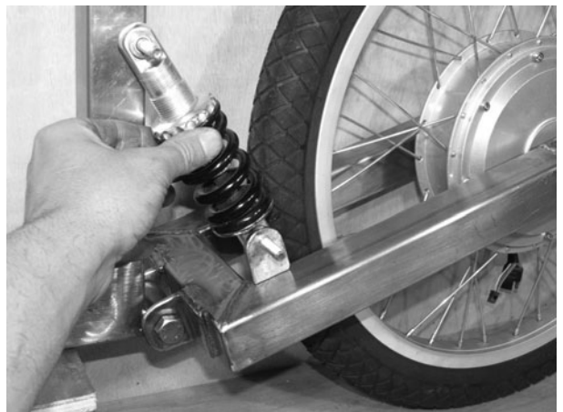
Figure 12-43 Determining the shock position
