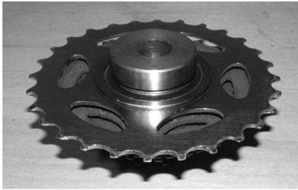
Figure 6-121 The freehub threads onto the machined part
