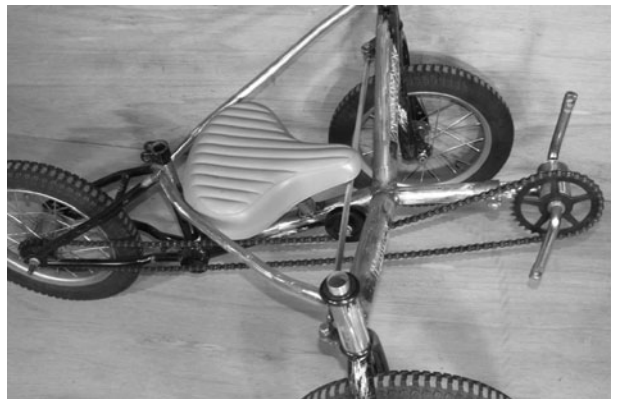
Figure 7-24 Adding the pilot's seat
