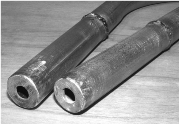
Figure 12-52 Capping the ends of the tubes
