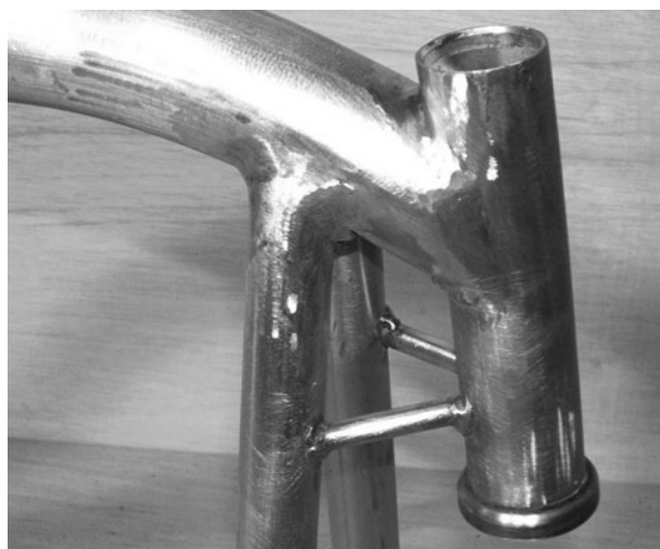
Figure 11-39 Head tube welded and gussets installed
