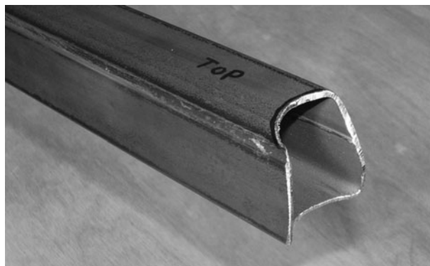
Figure 5-54 Adding the proper fish mouth to each end of the arm boom
