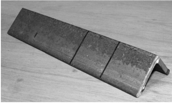
Figure 12-29 Cutting the rear dropouts
