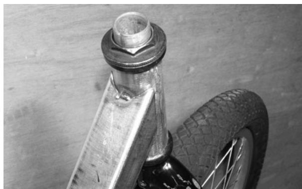
Figure 13-44 Tack welding the head tube in place
