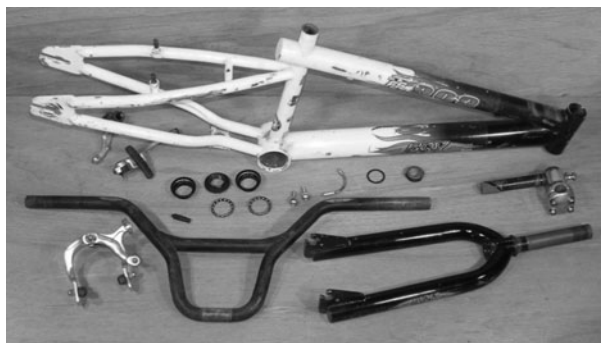
Figure 13-4 Taking everything apart for inspection
