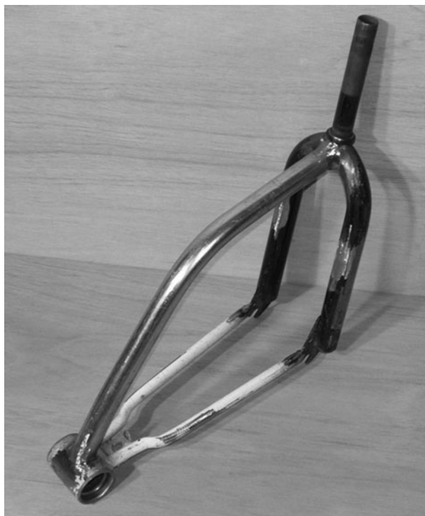
Figure 8-13 The fully welded and completed front end
