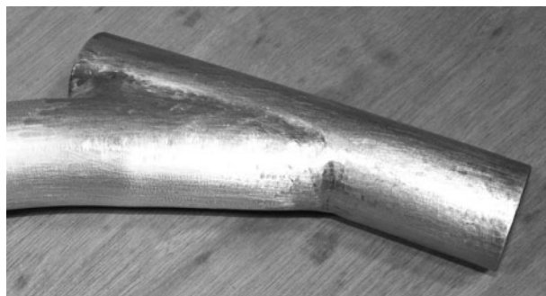
Figure 2-67 Cleaning up the beauty welds
