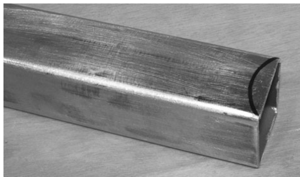
Figure 13-27 Making a cut for the bottom bracket
