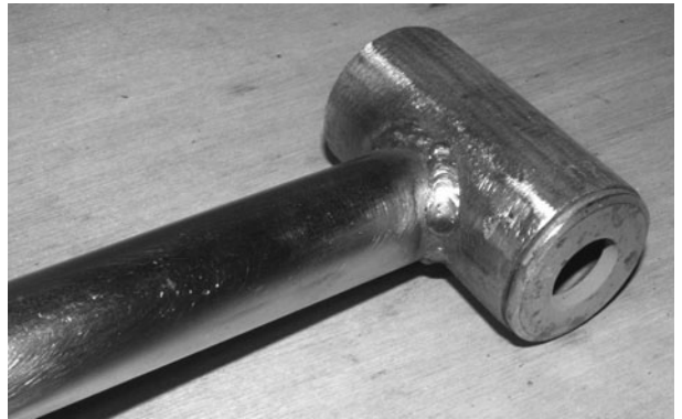
Figure 9-47 Bottom bracket welding completed
