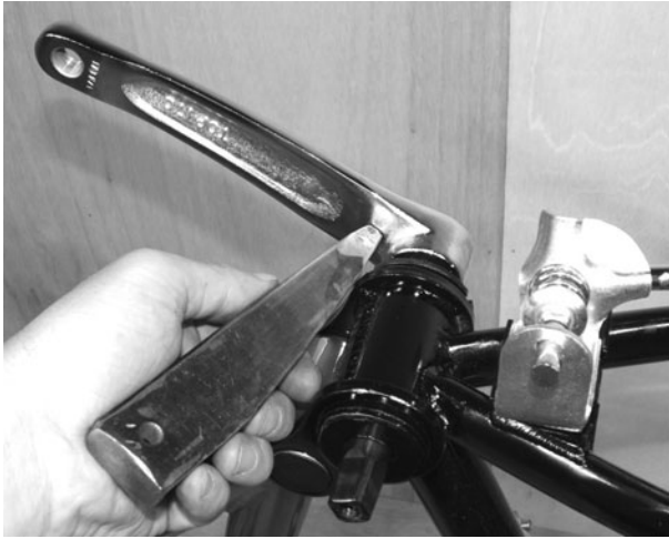
Figure 1-13 Removing the crank arm
