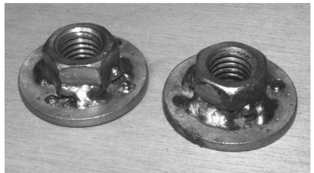
Figure 11-30 Weld the nuts to the washers
