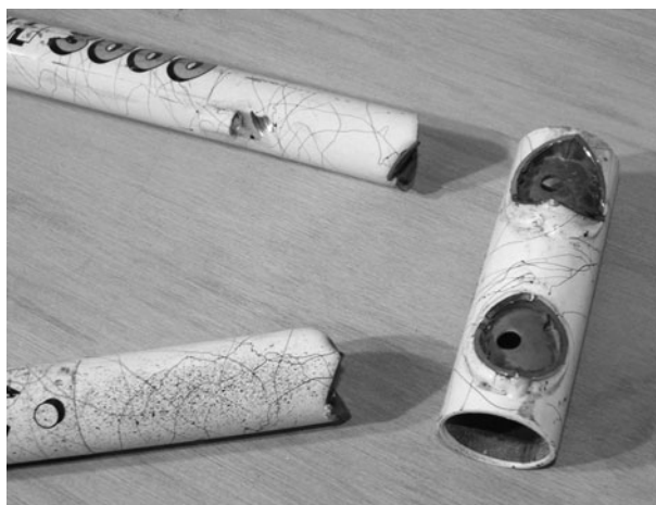
Figure 8-3 Removing the head tube from the rest of the frame
