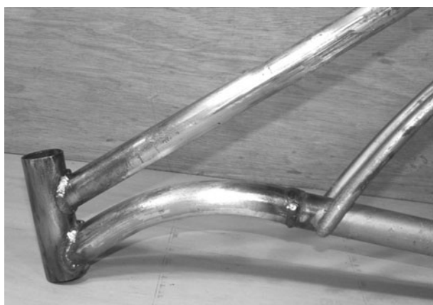
Figure 3-6 Adding the down tube extension
