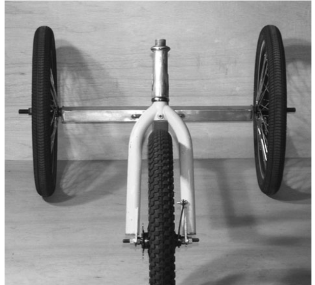
Figure 9-33 Checking head tube alignment
