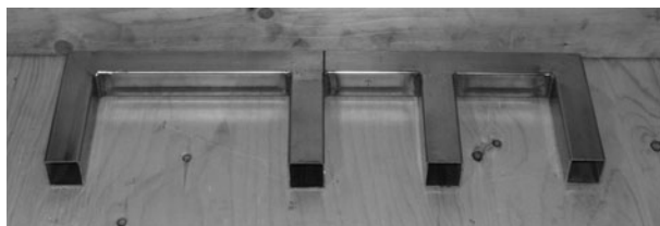
Figure 6-8 Completed rear frame section
