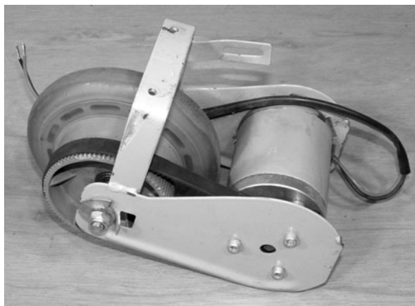
Figure 14-4 Scooter motor and drive wheel
