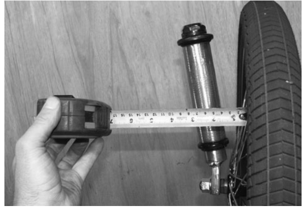
Figure 5-43 Measuring the head tube to tire center distance
