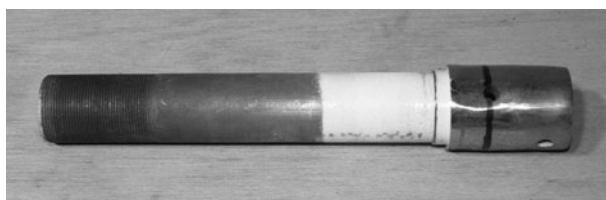
Figure 6-78 Remove the fork legs and grind the area
