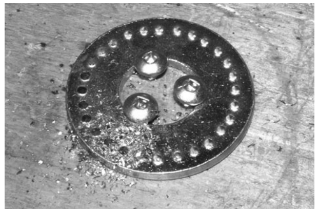
Figure 2-11 Bolting down the washer for drilling
