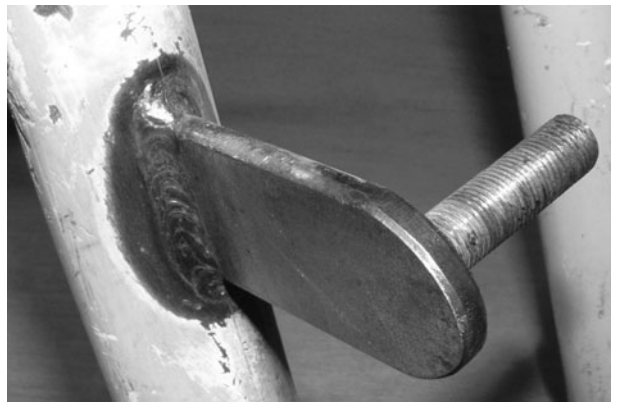
Figure 9-57 Mounting tab fully welded on both sides
