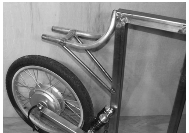
Figure 12-55 Completed seat mounting hardware
