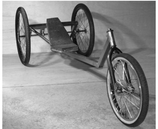
Figure 6-76 Finally, a rolling frame
