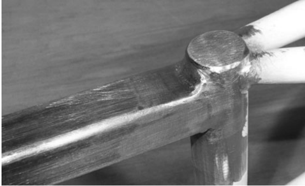
Figure 13-38 Seat tube cap completed
