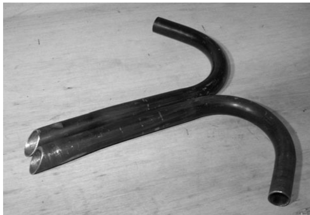
Figure 9-76 Leg mounting tubes cut to the same angle
