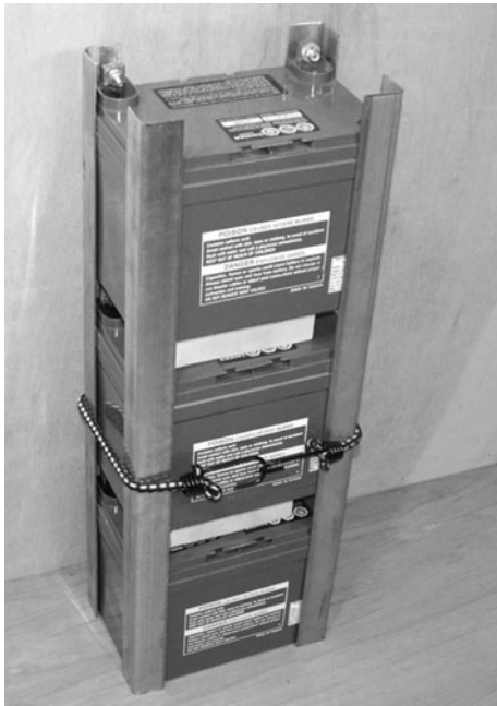
Figure 12-7 Battery pack side rails
