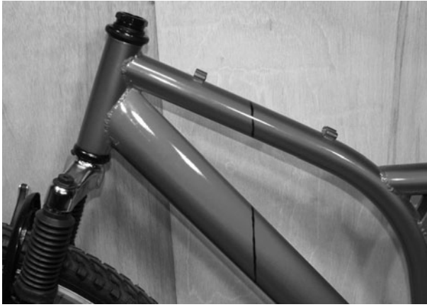
Figure 12-3 Marking the frame for cutting
