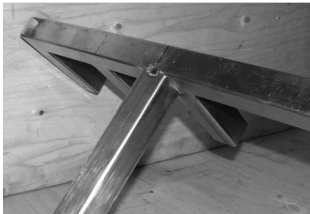
Figure 6-13 Joining the rear of the frame to the main frame
