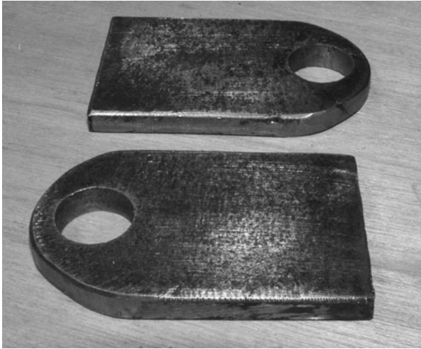
Figure 9-7 Drill the 14-mm axle holes
