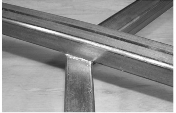
Figure 5-51 Welding the underside of the arm boom
