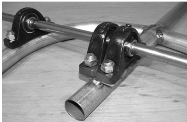
Figure 2-44 Welding the bearing mounting plate to the frame
