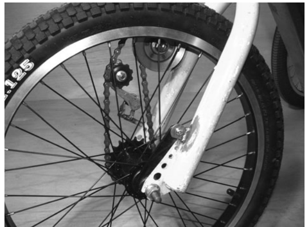
Figure 9-69 Brake mounting tab installed onto the fork leg
