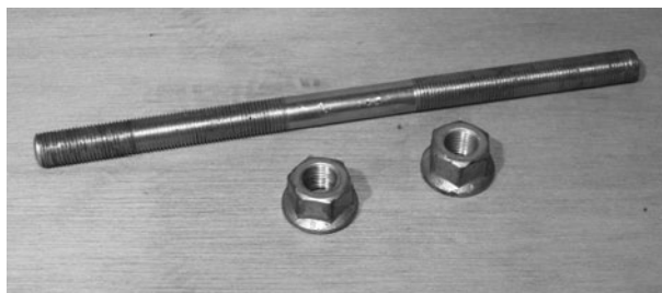
Figure 6-126 A rear hub axle will make a derailleur mounting peg
