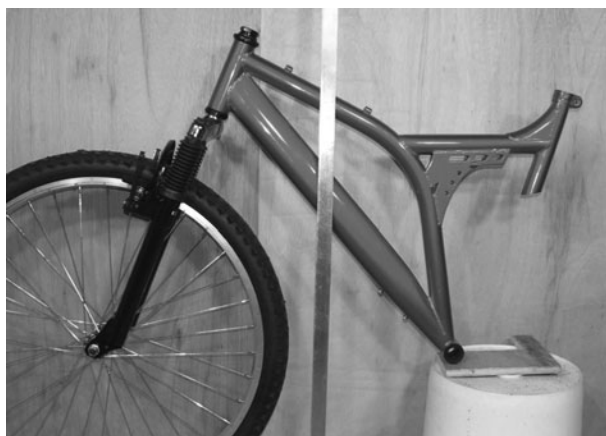
Figure 12-2 Using a guide bar to make a straight cut
