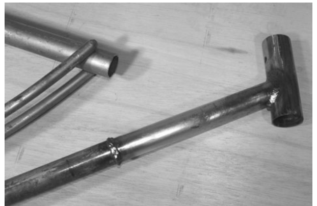
Figure 3-4 First tube completely welded
