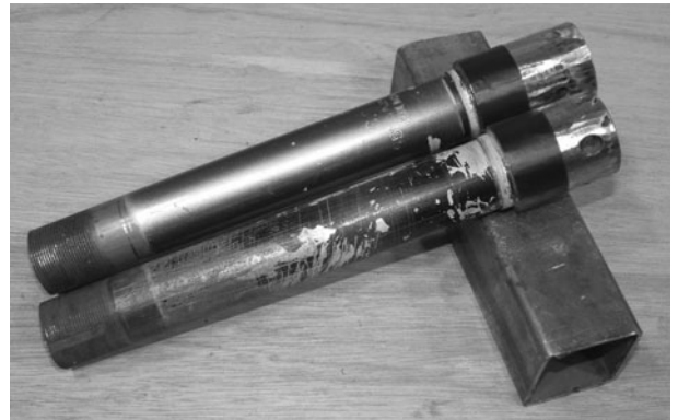
Figure 5-8 Cutting down the fork crowns
