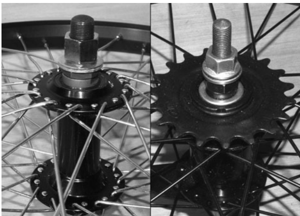
Figure 9-2 14-mm axle on the left; standard rear axle on the right
