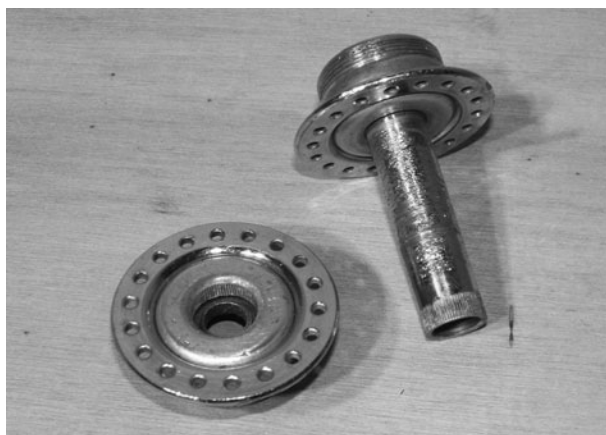
Figure 6-56 A steel hub can be taken apart
