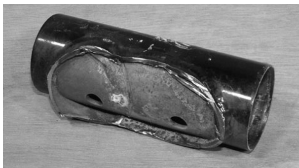
Figure 13-7 Cutting away the head tube
