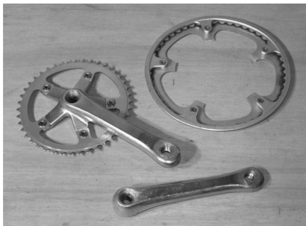
Figure 9-49 Reduce the crank set to a single gear
