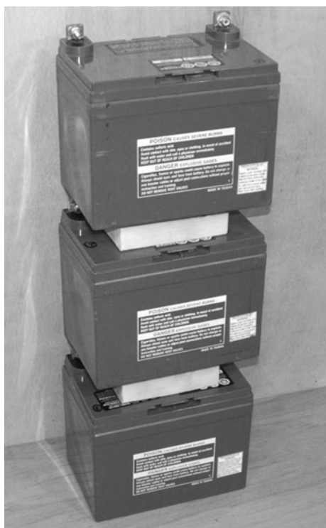
Figure 12-6 The mighty 36-volt stack
