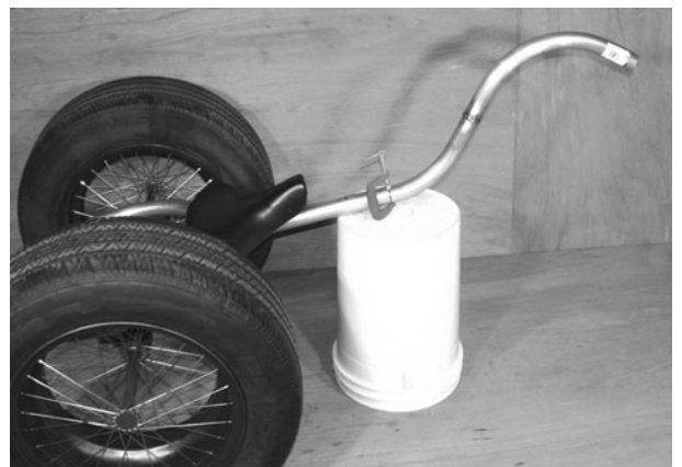
Figure 2-48 Joining the frame tubing
