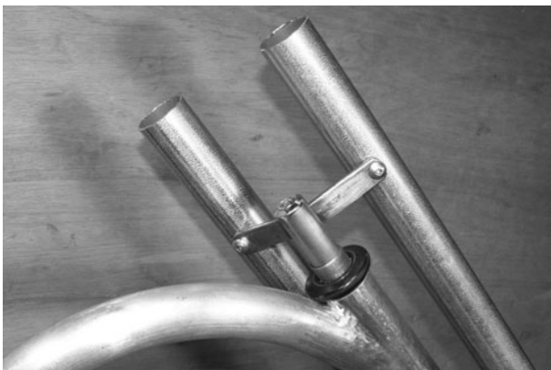
Figure 2-77 Front forks completed
