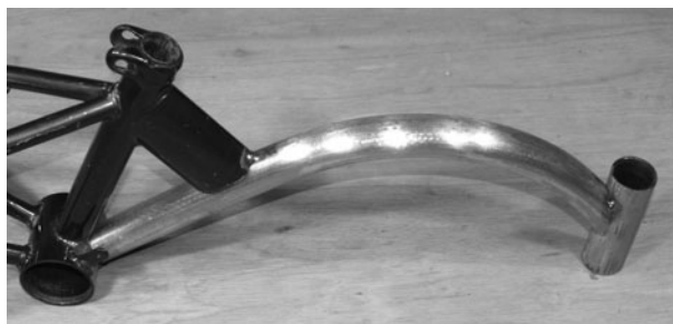
Figure 4-10 Tack welded frame
