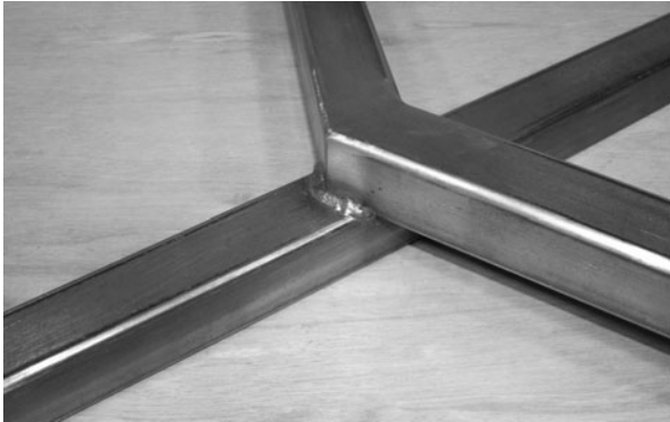
Figure 5-50 Welding the front arm boom to the main boom
