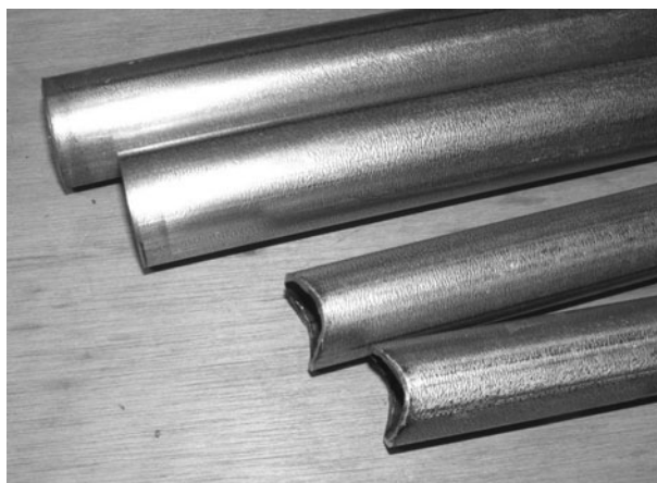
Figure 11-11 Preparing the down tubes and bottom tubes
