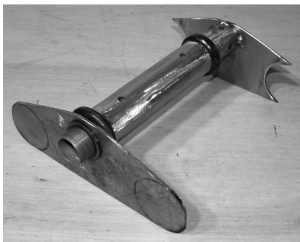
Figure 11-26 Tack welded triple tree
