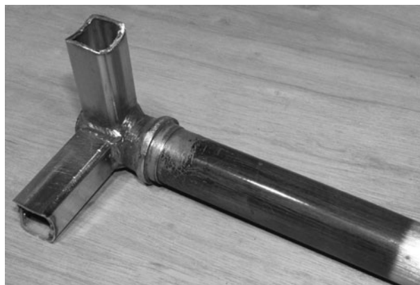
Figure 2-54 Fork leg support tubes welded in place
