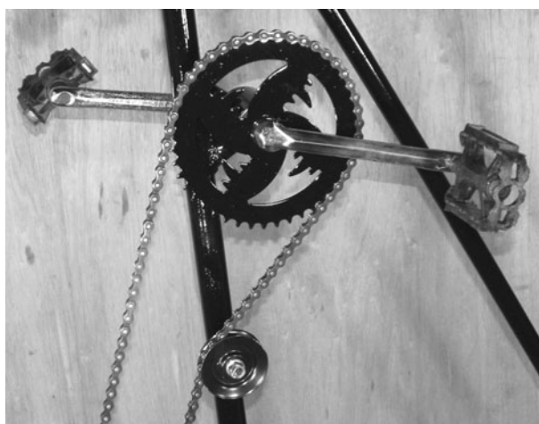
Figure 10-20 Installing the chain tensioner
