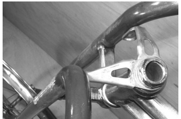
Figure 3-16 Top support brackets installed
