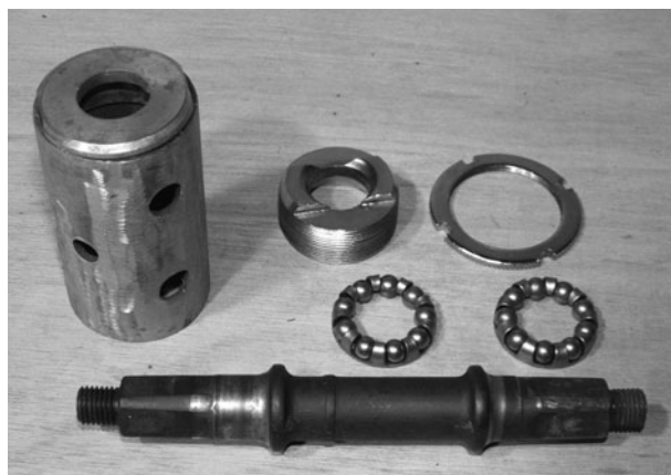
Figure 9-43 Bottom bracket cleaned up
