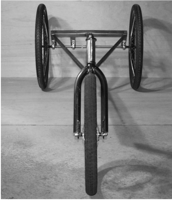
Figure 6-74 Checking head tube alignment
