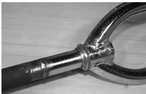
Figure 10-7 Welding the fork stem extension
