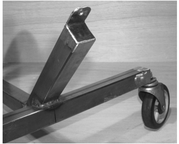
Figure 8-32 The rear seat mount also caps the open end of the tube
