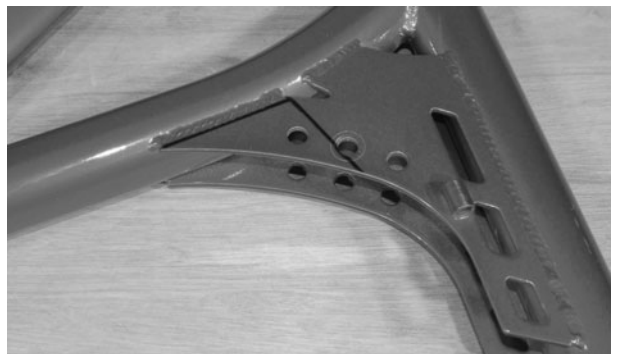
Figure 5-62 Salvaging the suspension mounting tabs
