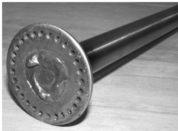
Figure 2-16 Outer hub flange welded to the axle
