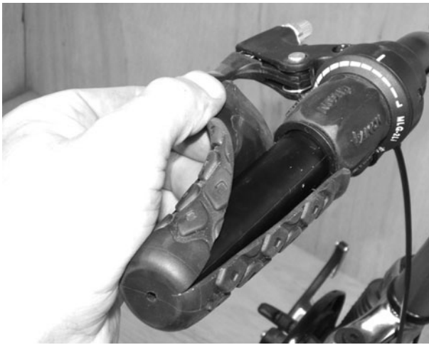
Figure 1-14 Removing old handle grips
