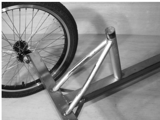
Figure 9-73 Welding the seat post to the frame
