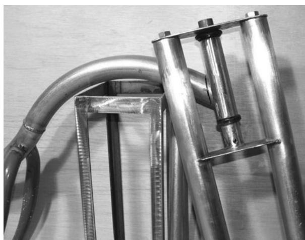
Figure 11-34 Marking the head tube angle cut
