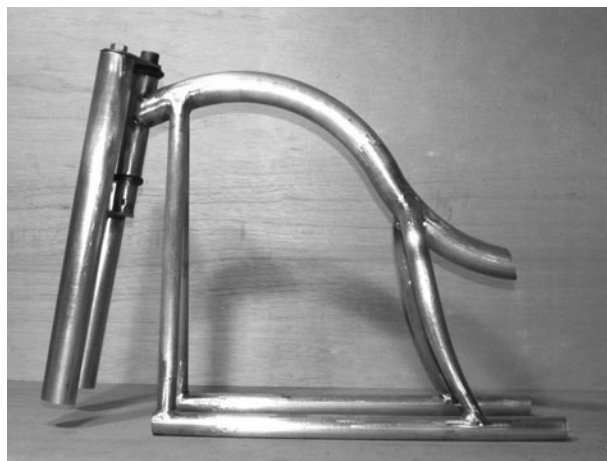
Figure 11-36 Tack welding the head tube in place
