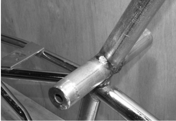
Figure 10-16 Foot peg position
