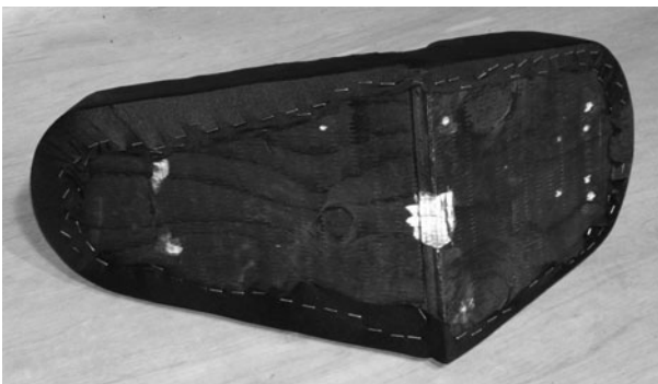
Figure 2-100 Seat material stapled in place
