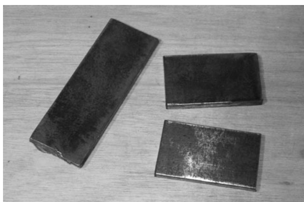
Figure 9-5 Cut two plates from the flat bar
