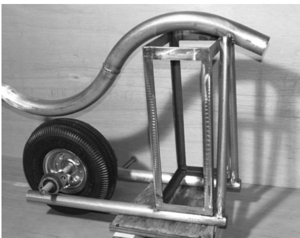
Figure 11-16 Installing one of the truss tubes
