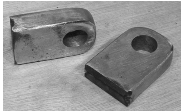
Figure 5-15 Finishing the \frac{9}{16} -inch axle holes
