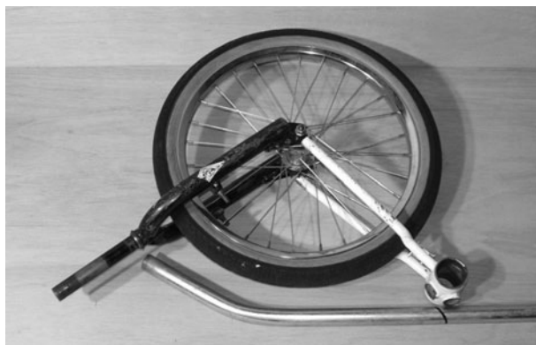
Figure 8-6 Laying out the front end parts
