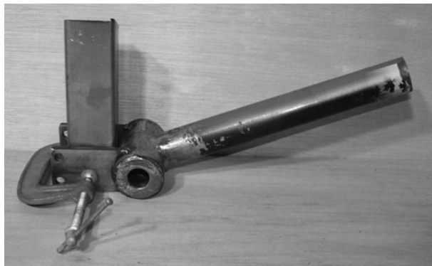
Figure 6-98 Using a bit of frame tubing as a welding guide
