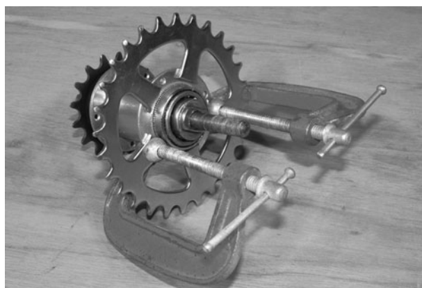
Figure 2-79 Adding the sprocket to the coaster shell
