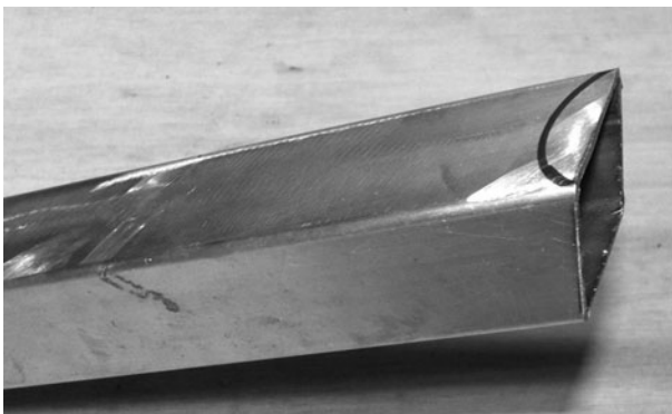
Figure 9-32 Grinding out the head tube joint
