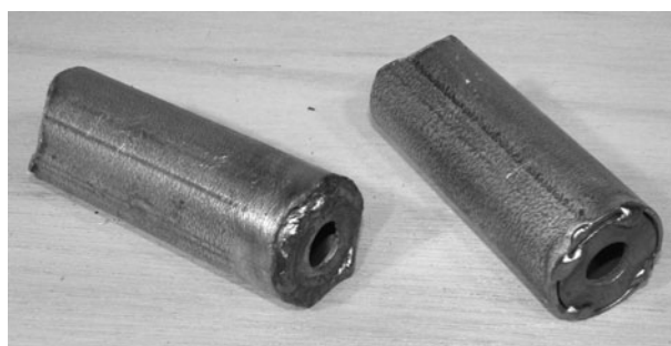
Figure 10-14 Poor man’s foot pegs
