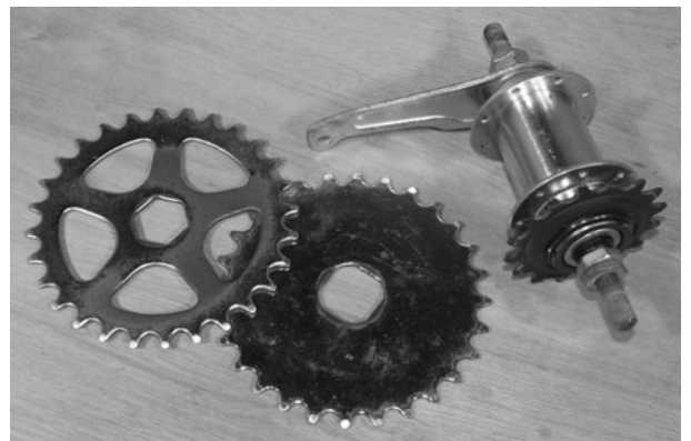
Figure 2-78 Mid-drive transmission parts
