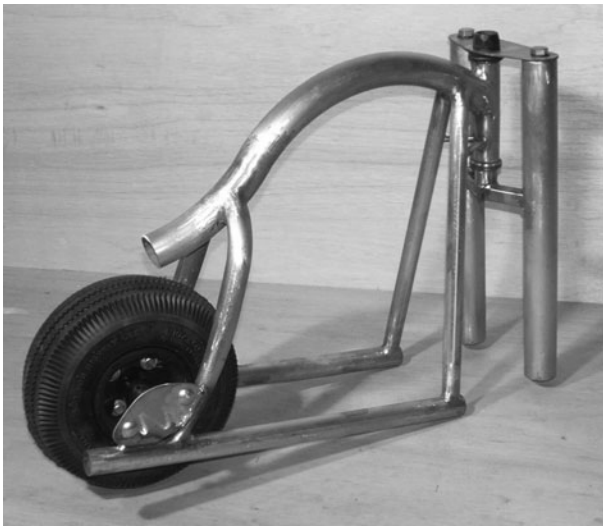
Figure 11-46 Bearing mounting plates installed
