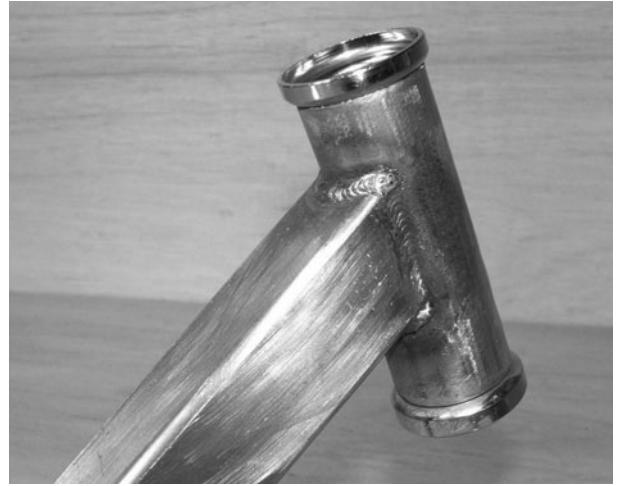
Figure 6-75 The head tube is fully welded
