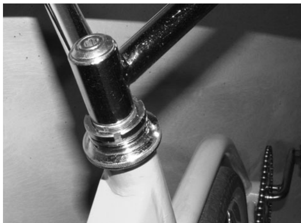
Figure 8-48 The gooseneck bolt must be very tight
