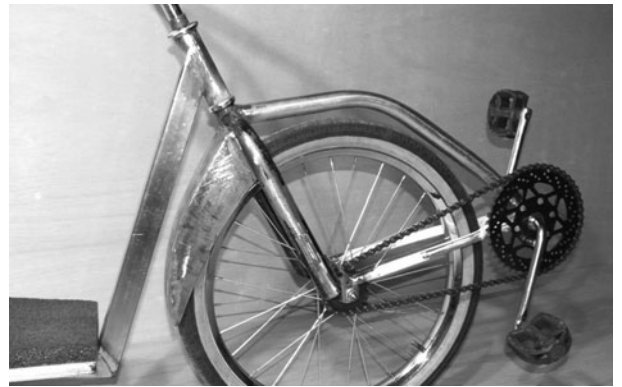
Figure 8-40 Optional but highly recommended fender installed
