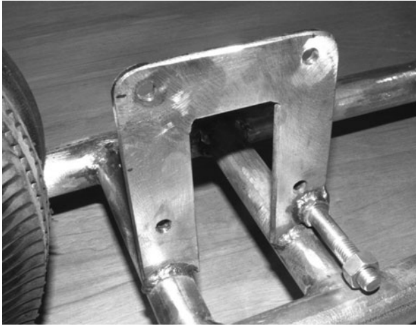
Figure 11-64 Idler pulley mounting bolt
