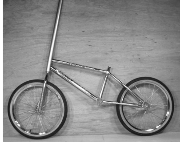
Figure 10-10 Installing the new tall head tube
