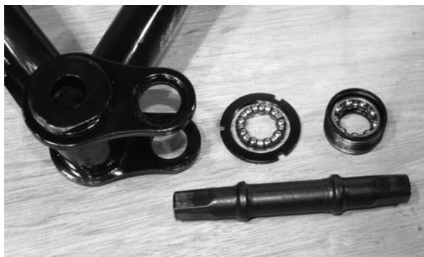
Figure 1-28 Removing the bottom bracket hardware
