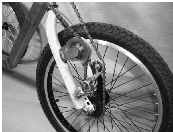
Figure 9-64 The return chain will be kept tight by the derailleur
