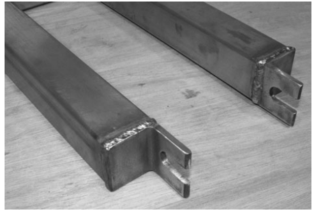
Figure 12-35 Completely welded dropouts
