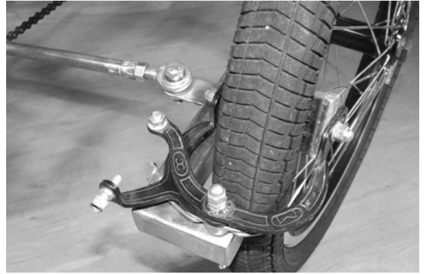
Figure 5-111 Installing the front brakes
