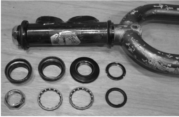
Figure 5-5 Checking the fork hardware
