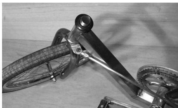
Figure 6-114 Steering at full left rotation
