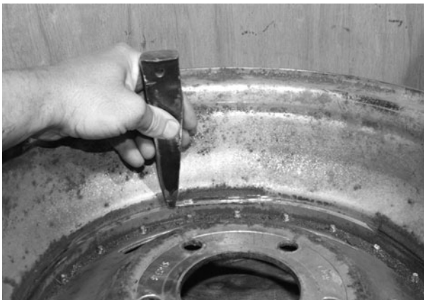
Figure 2-4 Pounding out the rim center
