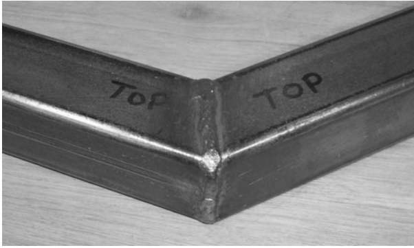
Figure 5-41 Front arm tubes joined
