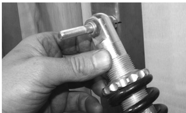
Figure 12-45 Marking the shock mounting bolts
