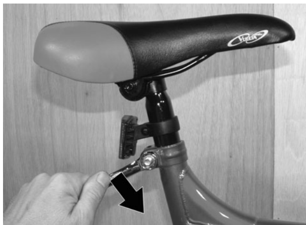
Figure 1-18 Removing the seat and seat post
