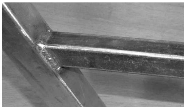
Figure 13-36 Welding the top tube to the front boom
