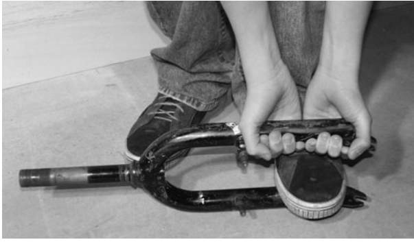
Figure 8-4 Opening the front forks to take the rear wheel
