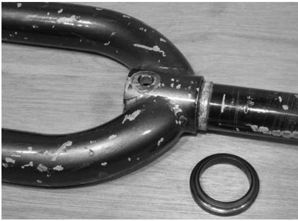
Figure 5-6 Remove the bearing race before cutting the fork legs
