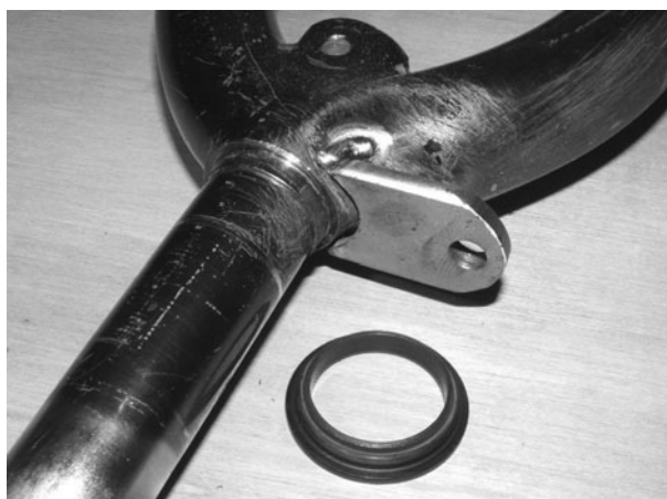
Figure 6-107 Make a tack weld at one end only
