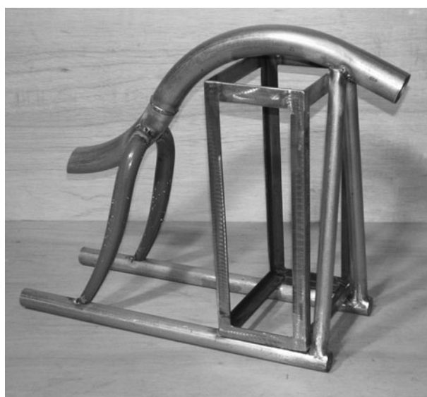
Figure 11-20 Tack welding the frame tubing
