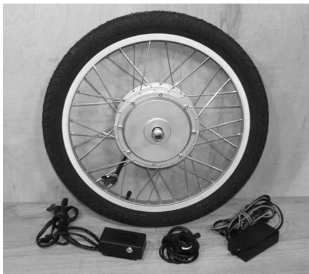
Figure 12-23 A complete hub motor kit
