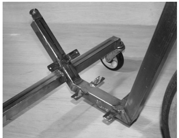
Figure 8-34 The other seat mounts are welded to the frame
