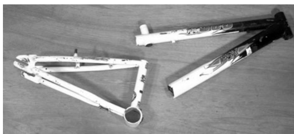
Figure 13-5 Cutting away the rear triangle
