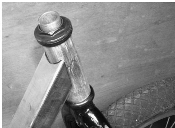
Figure 13-43 Checking the head tube angle
