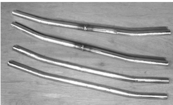
Figure 7-13 Joining the seat stays to make two longer tubes
