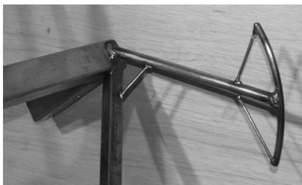
Figure 6-139 Completed elbow guards
