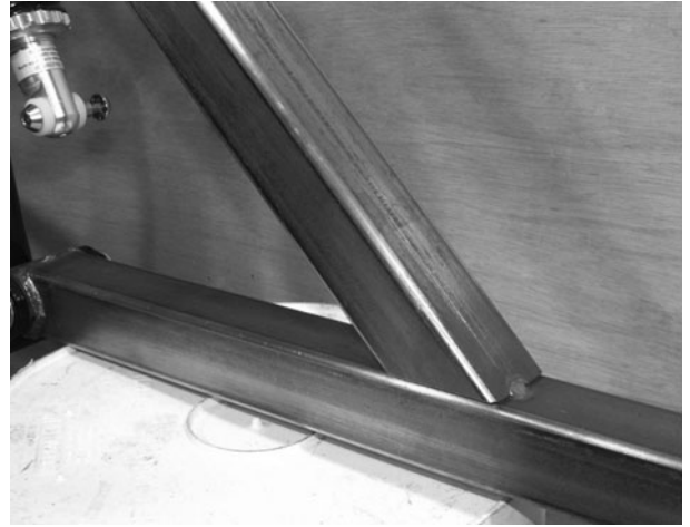
Figure 5-35 Tack welded seat tube
