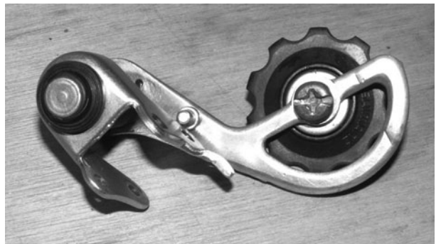
Figure 9-62 Bolt the small derailleur wheel in place
