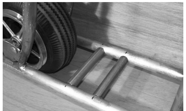
Figure 11-55 Motor mounting plates installed
