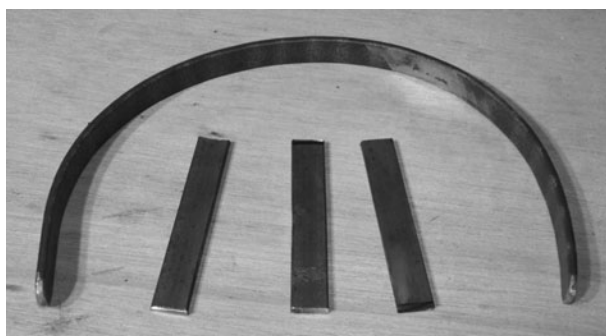
Figure 9-79 Some half-inch flat bar bent around the front chain ring
