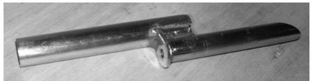
Figure 9-41 Gooseneck extension fully welded
