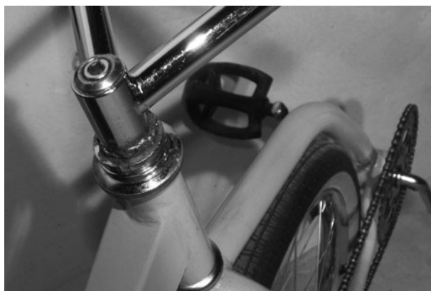
Figure 8-49 This gooseneck will never move out of alignment now
