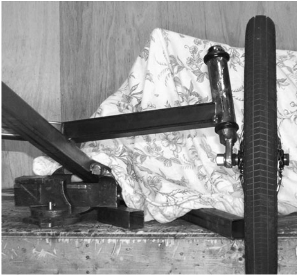
Figure 5-57 Welding the head tube in place
