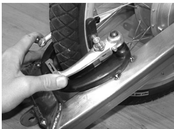
Figure 12-59 Mounting the rear brakes
