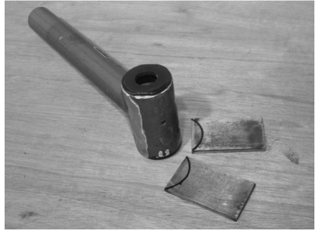
Figure 5-84 Creating an adjustable bottom bracket
