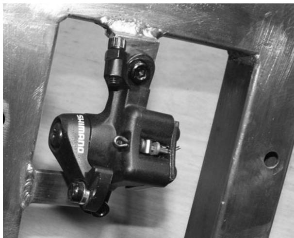
Figure 6-145 Disc brake mounts securely welded
