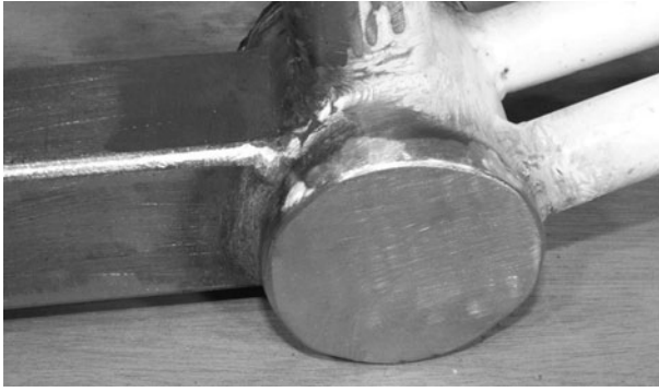
Figure 13-53 Grinding the caps clean
