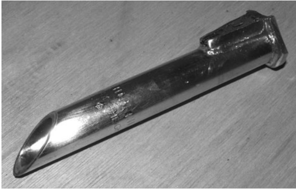
Figure 9-38 Cut the top from the gooseneck
