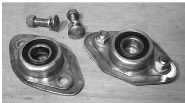
Figure 11-43 Both bearing plates ready for mounting
