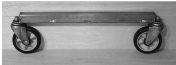
Figure 8-17 Mounting the caster wheels to the rear T-bar
