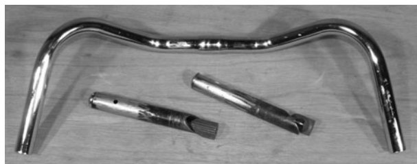
Figure 5-100 Trimmed goosenecks and a bicycle handlebar
