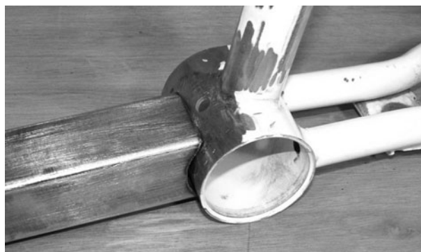
Figure 13-28 Checking the bottom bracket joint
