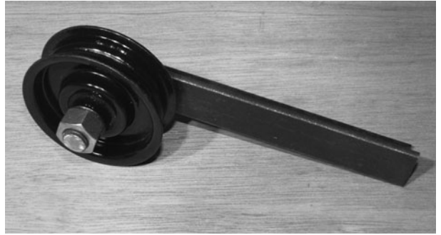
Figure 11-66 Idler pulley installed
