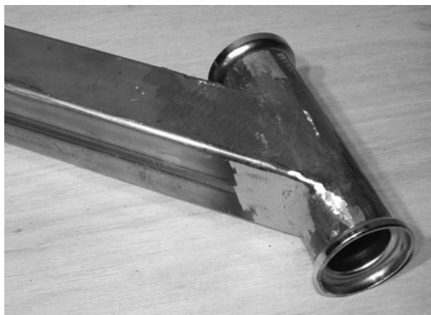
Figure 8-23 Welded and ground joint between front tube and head tube
