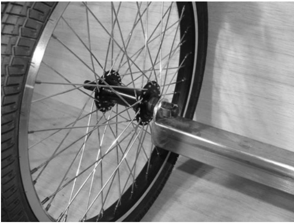
Figure 9-12 Checking rear wheel alignment
