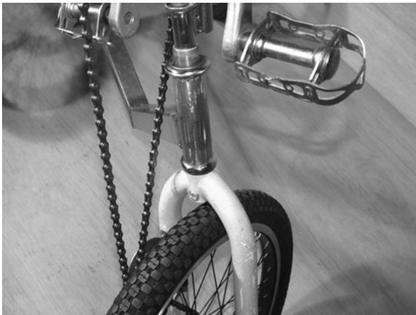
Figure 9-67 The chain will not rub on the frame during normal use
