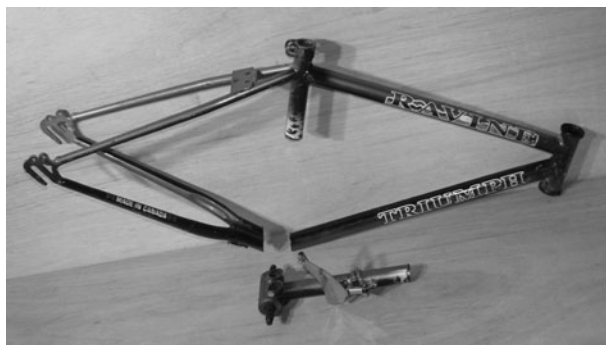
Figure 6-92 Cut the bottom bracket and seat tube from the donor frame
