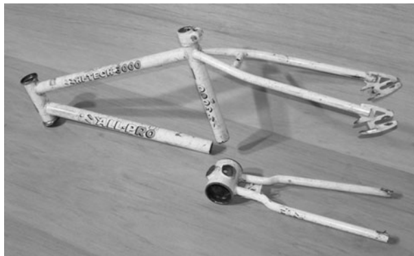
Figure 8-2 Cut the chain stays and bottom bracket from the frame
