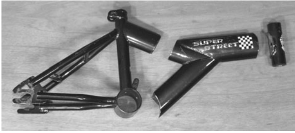
Figure 4-3 Hacking up the frame
