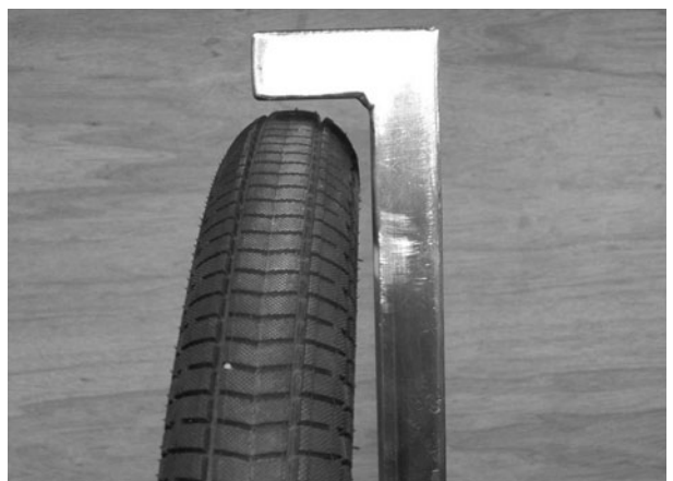
Figure 5-70 Checking brake arm clearances
