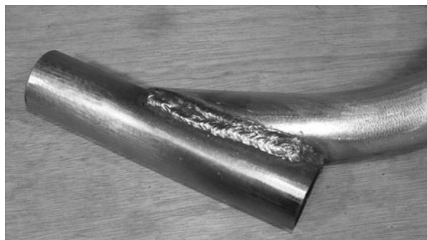
Figure 2-66 Completing the head tube welds
