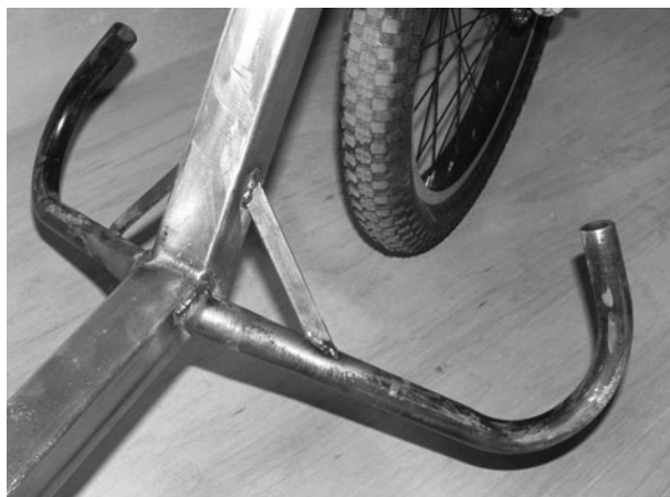
Figure 9-78 Leg mount support gussets
