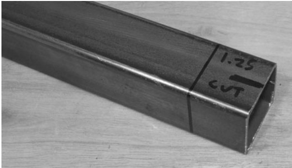
Figure 5-46 Trimming the front arm boom assembly
