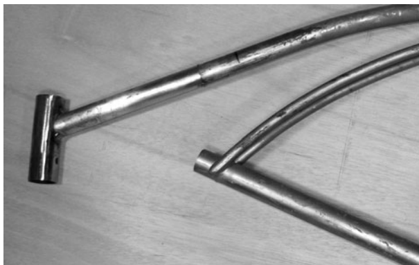
Figure 3-3 Installing the top tube extension
