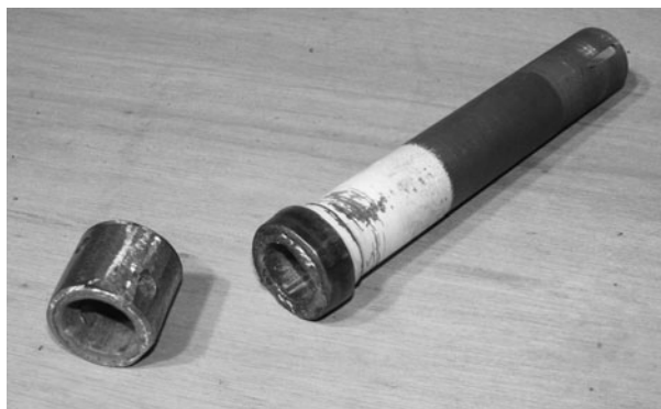
Figure 6-79 Cut and secure the crown together by welding
