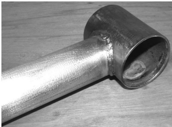
Figure 2-70 Bottom bracket welding completed
