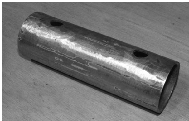
Figure 9-27 Head tube ground clean
