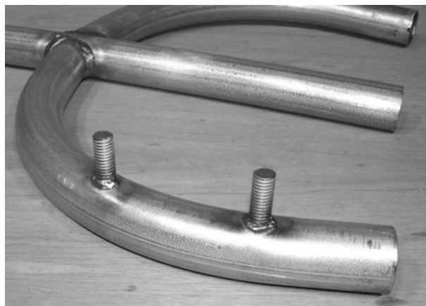
Figure 2-42 Bolts welded directly to the frame
