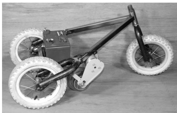
Figure 14-14 Drive motor installed
