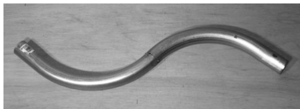
Figure 11-8 Elbows tack welded together
