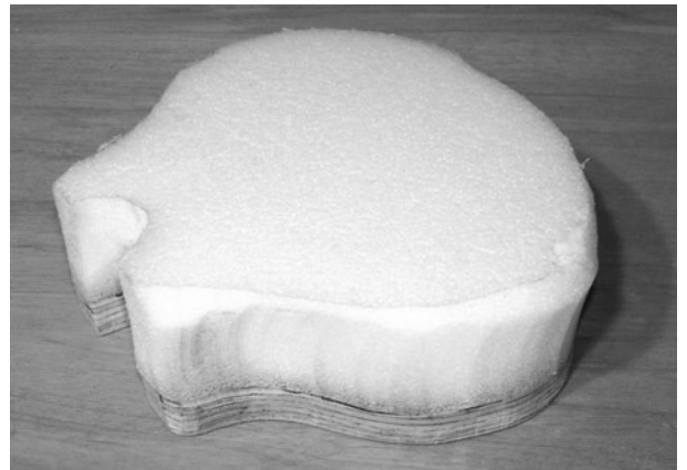
Figure 11-80 Foam trimmed and glued to the wood
