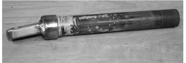
Figure 5-18 Mounting the axle tabs to the fork stem
