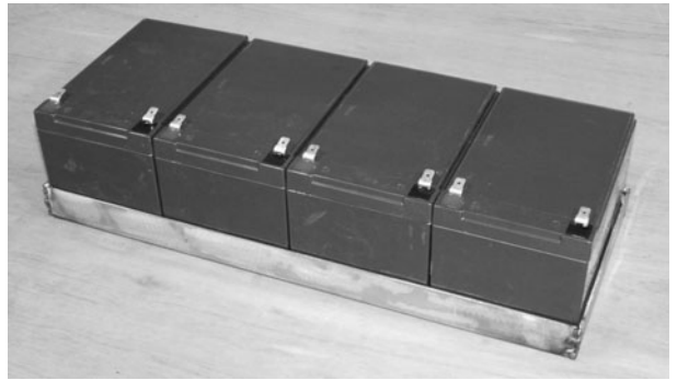
Figure 13-14 Test fitting the batteries in the frame
