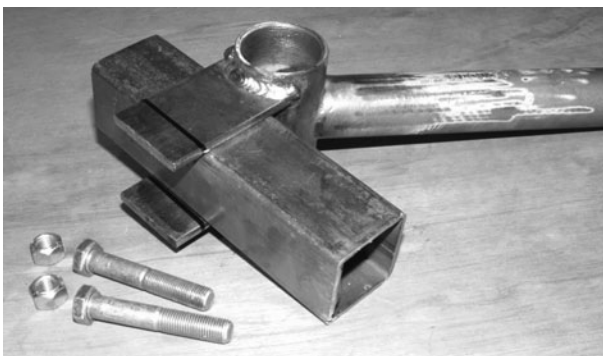
Figure 5-90 Marking a line to drill the bolt holes
