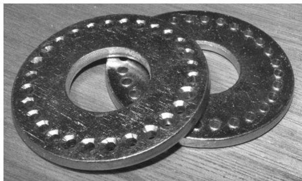
Figure 2-12 Beveling each spoke hole
