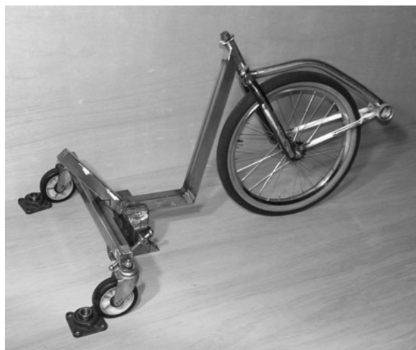
Figure 8-25 Determining the proper T-bar to frame placement
