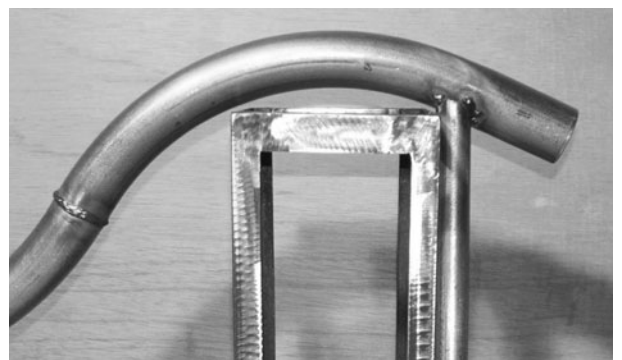
Figure 11-17 Tack welding the frame together
