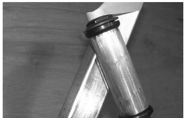
Figure 13-41 Marking the line to cut the boom
