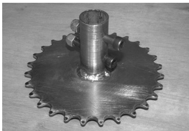
Figure 2-83 Rear-drive axle sprocket completed
