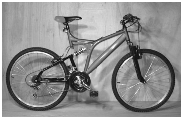
Figure 1-1 A typical all-steel suspension mountain bicycle
