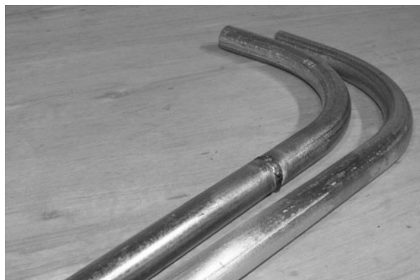
Figure 2-89 Weld and grind to hide seams
