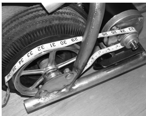
Figure 11-69 Measuring the belt size
