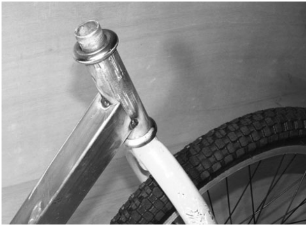
Figure 9-34 Tack weld the head tube
