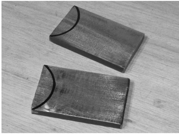
Figure 6-95 Bottom bracket plates ready to be ground
