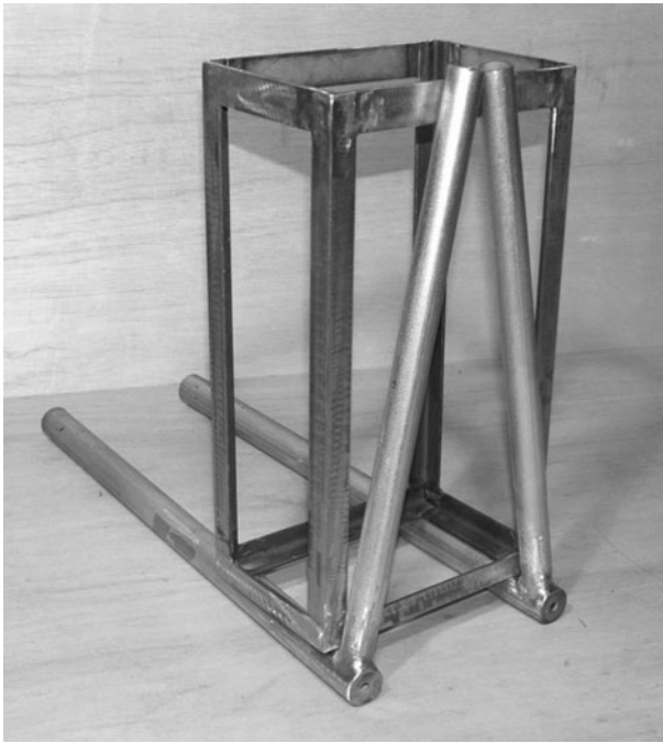
Figure 11-15 Laying out the frame tubing
