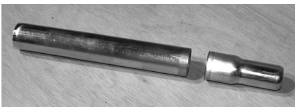
Figure 9-39 A seat post will be used to lengthen the neck
