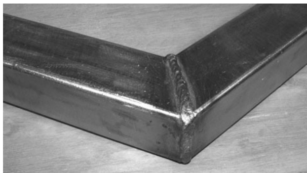
Figure 13-25 Side boom joint completed
