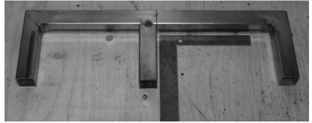
Figure 6-6 Installing the drive-side axle mount tube
