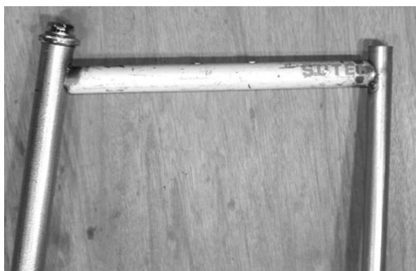
Figure 10-12 Adding the new top tube
