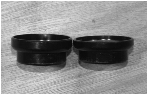
Figure 1-23 Head tube cups have a top and bottom
