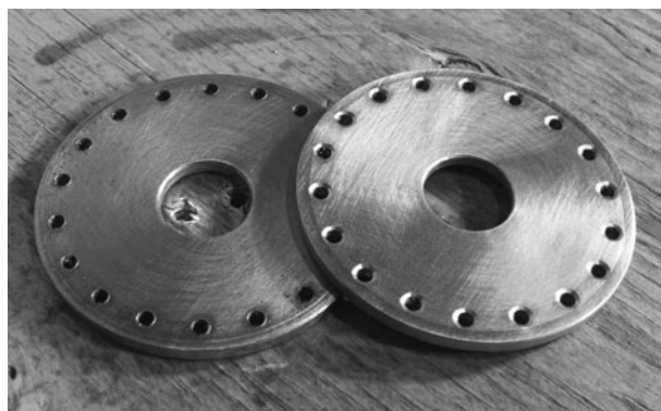
Figure 6-33 Drilled (left) and beveled (right)
