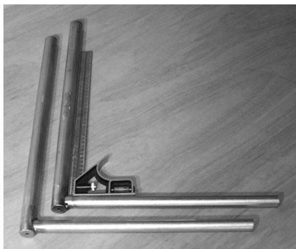
Figure 11-14 Joining the down tubes and bottom tubes at 90 degrees
