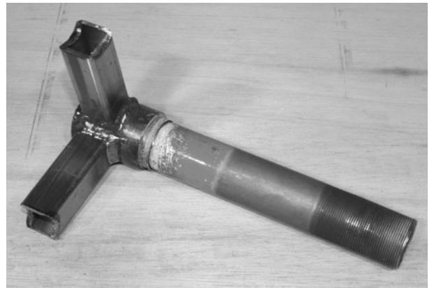
Figure 3-12 Fork tubing welded
