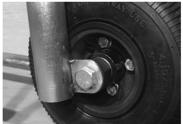
Figure 11-48 Front axle installed with a temporary spacer
