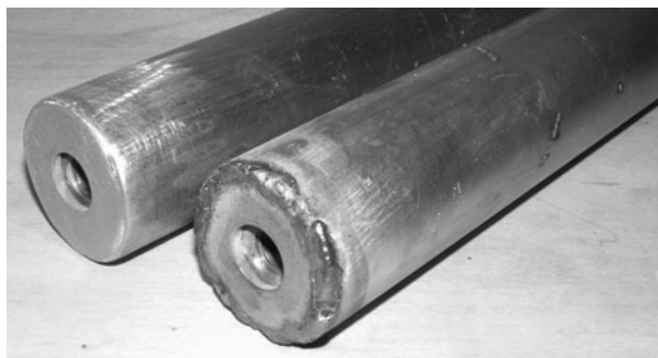
Figure 11-31 Welding the washers to the top of the fork tubing
