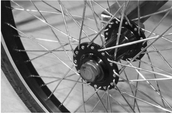
Figure 9-82 Trim away the outer axle stubs
