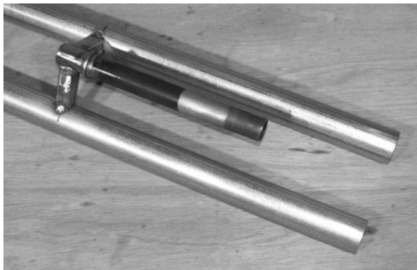
Figure 2-56 Welding the fork stem in place
