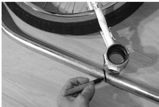
Figure 8-7 Marking the steering boom to be cut
