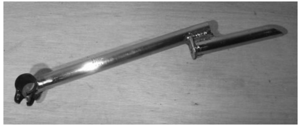
Figure 6-103 The handlebar clamp is in the center of the gooseneck tube
