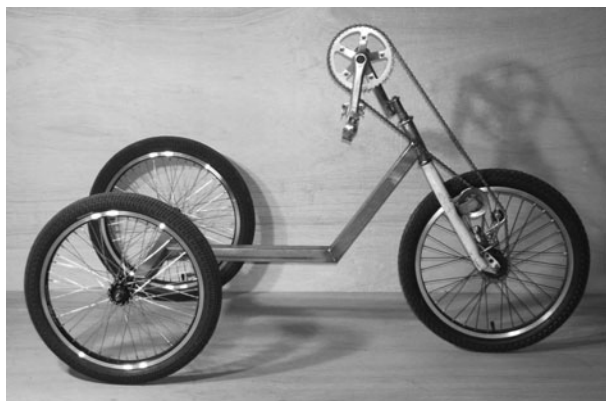
Figure 9-70 Transmission and brakes completed
