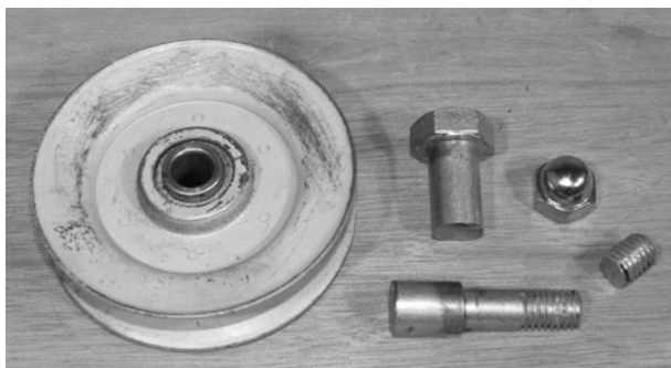
Figure 5-94 A V-belt idler will guide the chain around the frame
