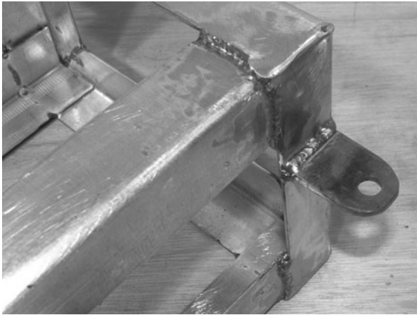
Figure 12-48 Installing the battery pack tabs
