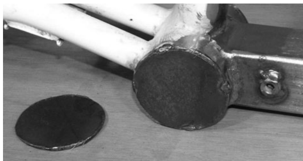
Figure 13-61 Capping off the open bottom bracket
