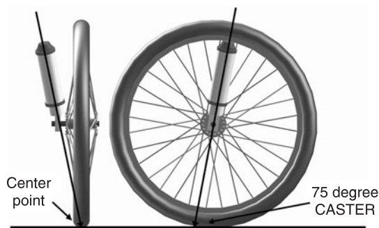
Figure 5-53 Head tube angles of concern
