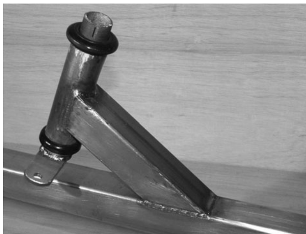
Figure 6-90 Steering support tube completely welded
