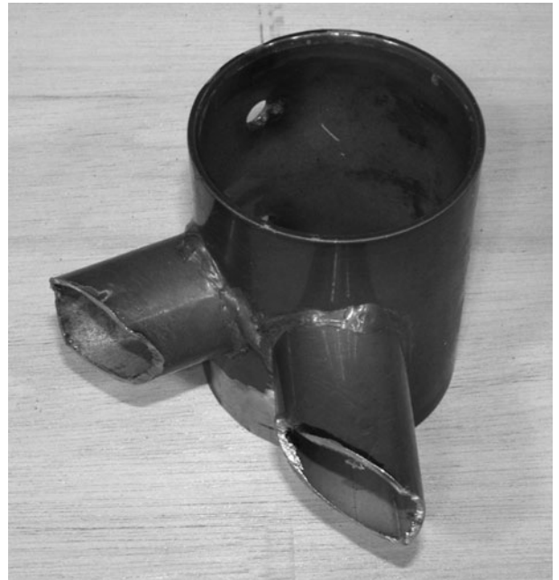
Figure 10-17 Adding the bottom bracket
