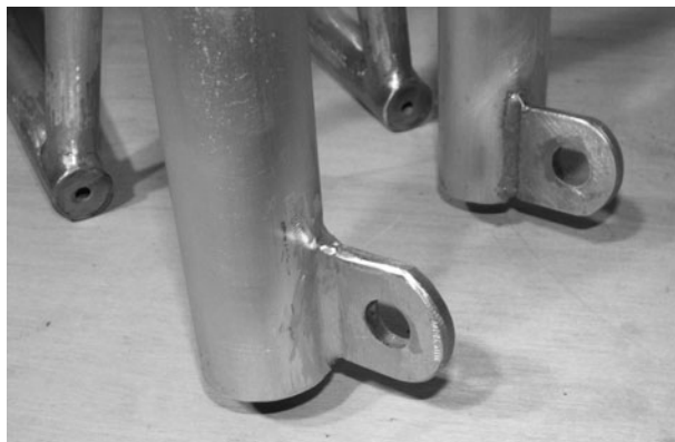
Figure 11-50 Fork dropouts welded in place
