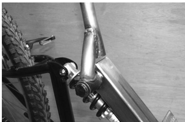
Figure 5-107 Installing the adjustable backrest
