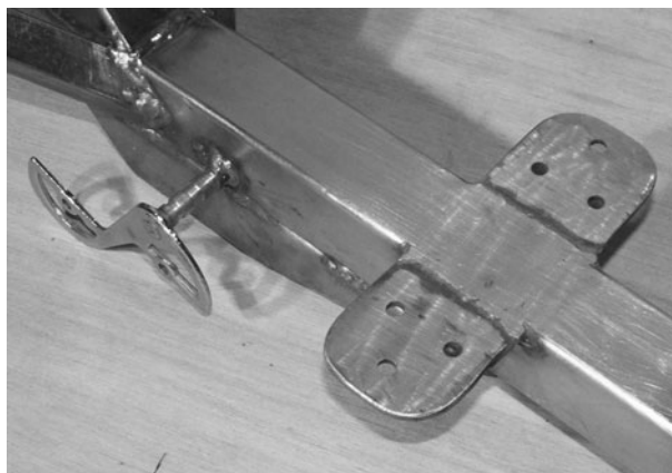
Figure 6-147 Seat mounts welded to the main boom
