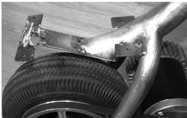
Figure 11-73 Seat mounting plates installed
