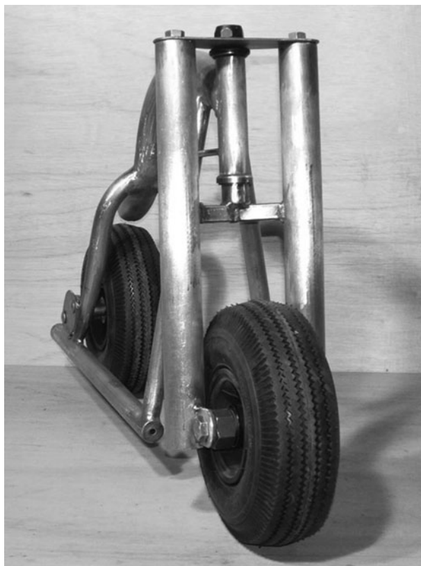
Figure 11-49 Checking front wheel alignment
