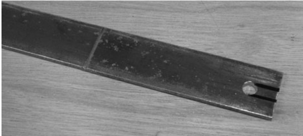
Figure 13-17 Making the slotted hole
