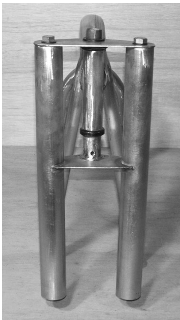
Figure 11-37 Checking head tube alignment
