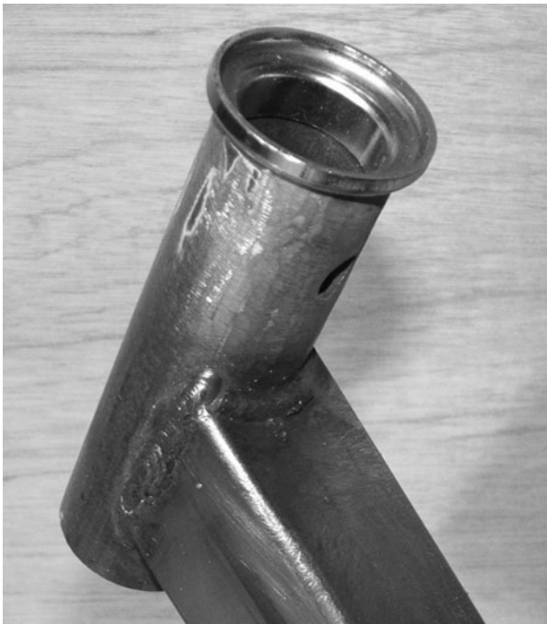
Figure 9-35 Completed head tube welding
