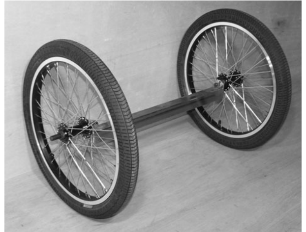
Figure 9-13 Both rear wheels should be parallel
