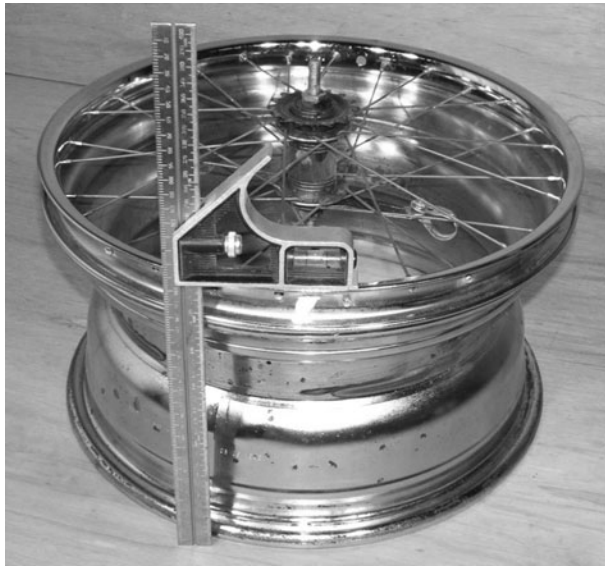
Figure 2-20 Marking the rims' spoke holes
