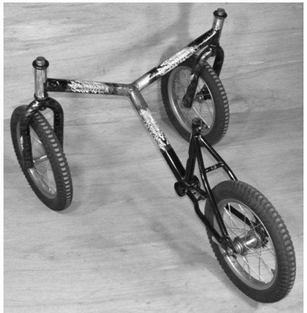
Figure 7-11 Tack welding the front and rear of the trike frame
