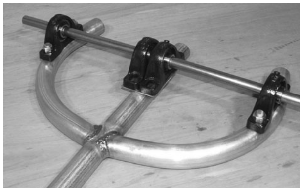
Figure 2-43 Aligning the two inner bearings
