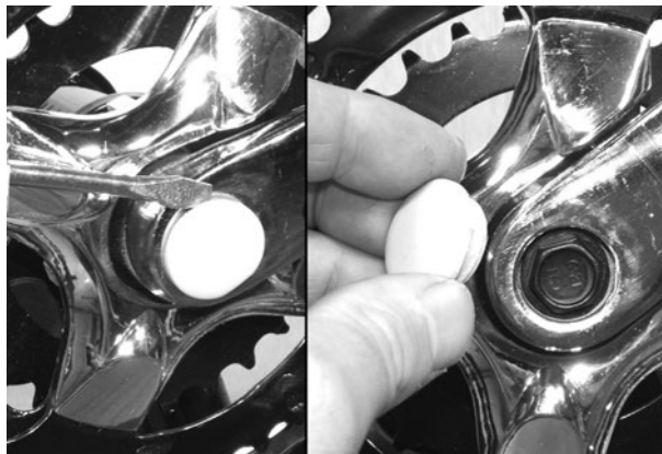
Figure 1-11 Removing the crank arms
