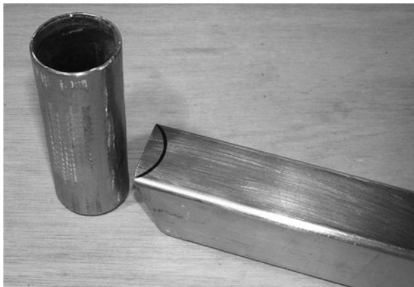
Figure 6-67 Tracing the area to be ground out
