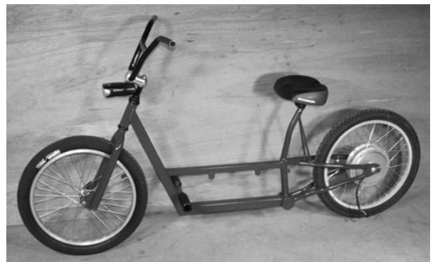
Figure 13-66 The basic rolling chassis painted
