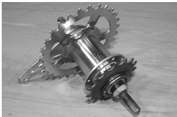
Figure 2-81 Sprocket added to the coaster shell
