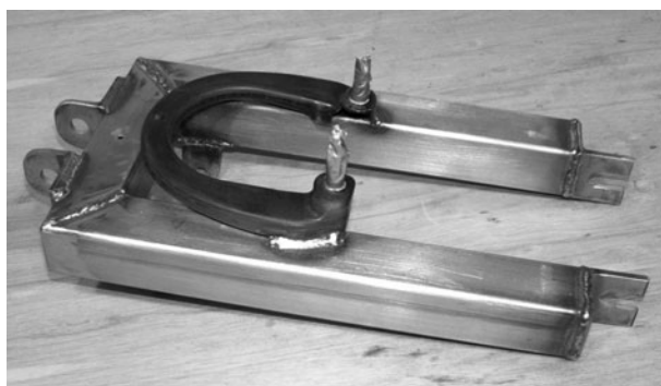
Figure 12-60 Rear brake assembly installed
