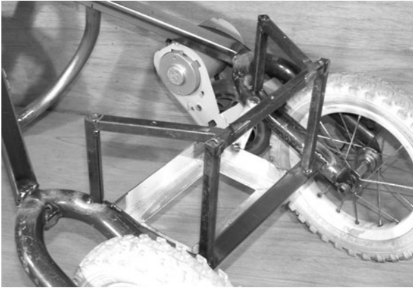
Figure 14-17 Installing the seat frame
