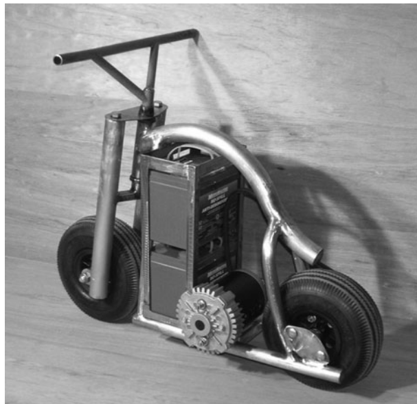
Figure 11-60 The battery box test fit
