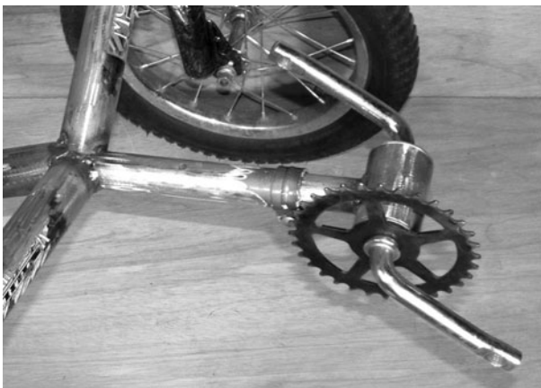
Figure 7-18 Installing the bottom bracket boom
