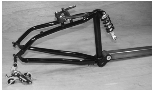
Figure 5-29 Rear triangle installed onto the main boom
