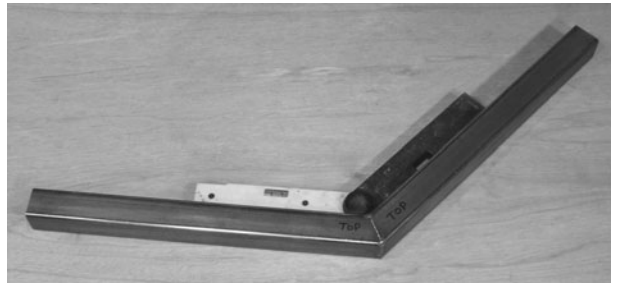
Figure 5-39 Joining the two front arm tubes
