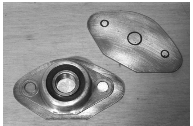
Figure 11-41 Making the bearing mounting plates
