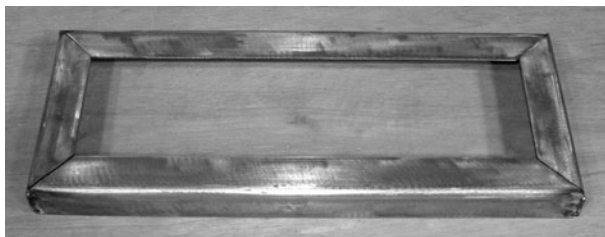
Figure 13-13 Battery pack base tack welded
