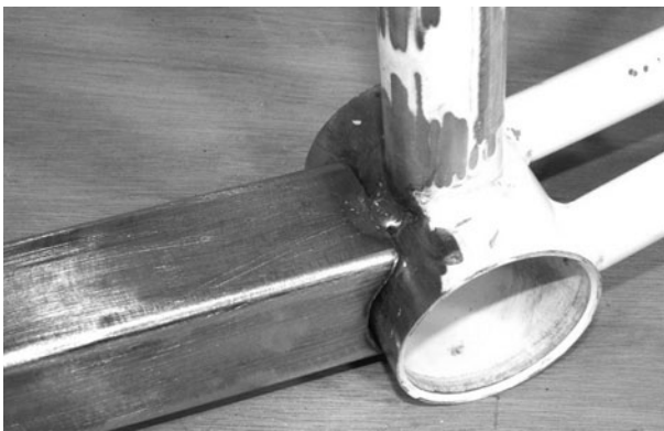
Figure 13-30 Boom and bottom bracket tack welded
