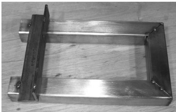
Figure 12-27 Tack welding the swingarm tubes
