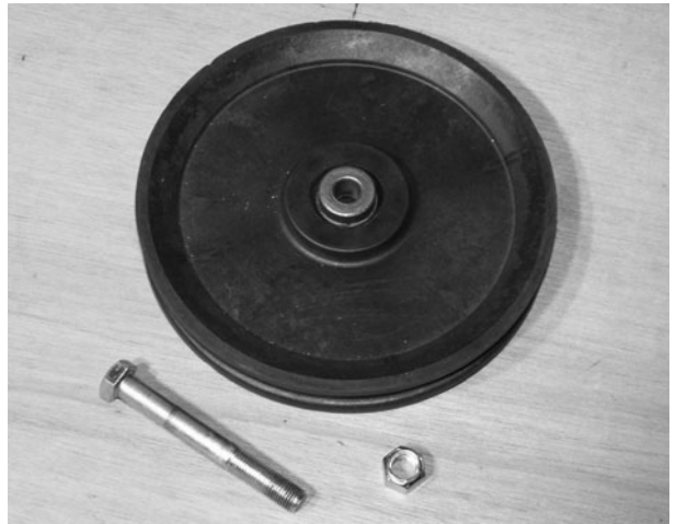
Figure 6-116 A nylon idler pulley with ball bearing
