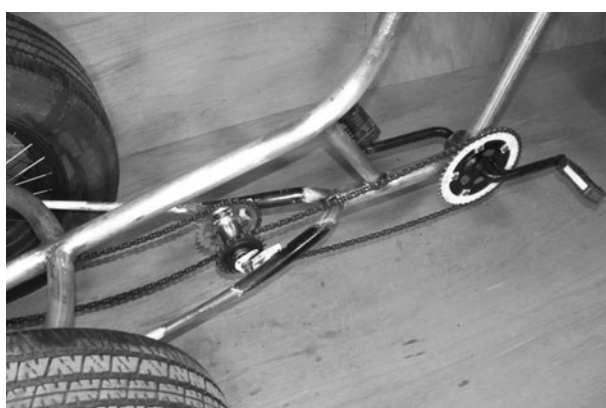
Figure 2-86 Installing the mid drive
