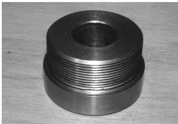
Figure 6-120 Machined version of the freehub mounting part
