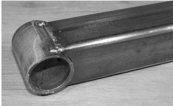
Figure 5-27 Pivot tube tack welded in place
