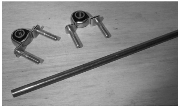
Figure 6-34 One of the rear axles and a set of pillow block bearings
