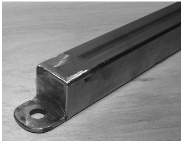
Figure 8-19 The completed T-bar fully welded and ground smooth
