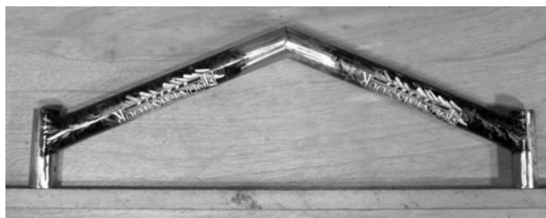
Figure 7-6 Joining the head tubes
