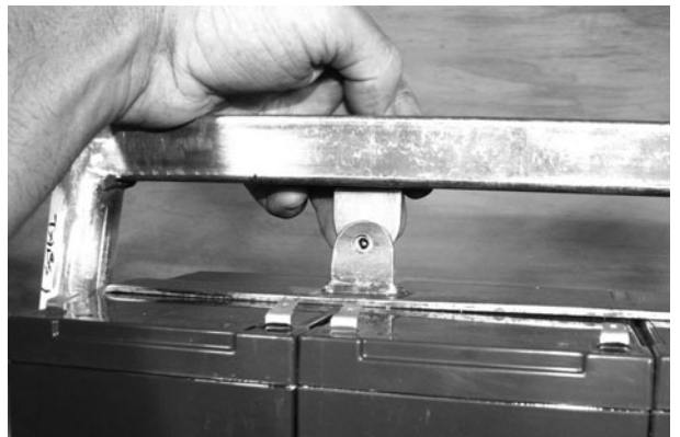
Figure 13-53 Installing the upper battery box tabs
