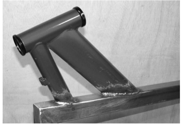
Figure 12-22 Front frame completely welded
