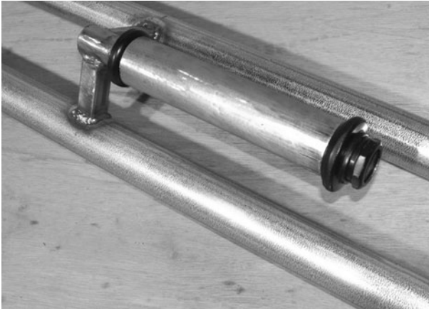
Figure 2-59 Fork hardware installed
