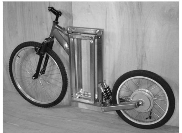
Figure 12-50 Battery pack fully installed
