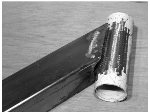
Figure 8-21 Cutting the front tube to mate with the head tube
