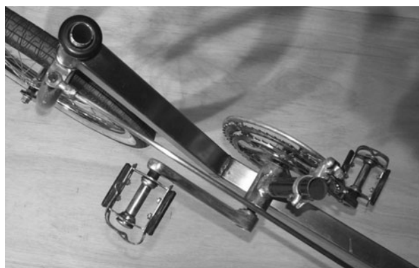
Figure 6-115 The control rod has plenty of room
