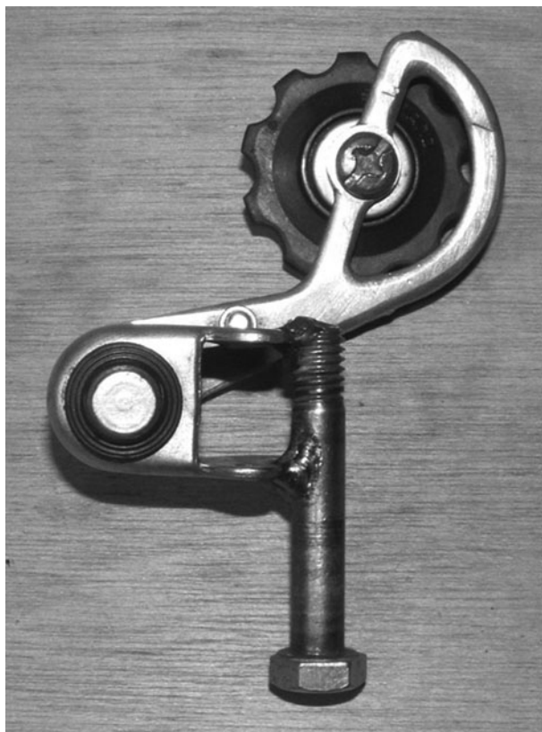
Figure 9-63 Mounting post installed onto the derailleur
