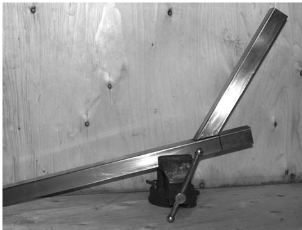
Figure 6-11 Getting ready to join the main boom and seat tube
