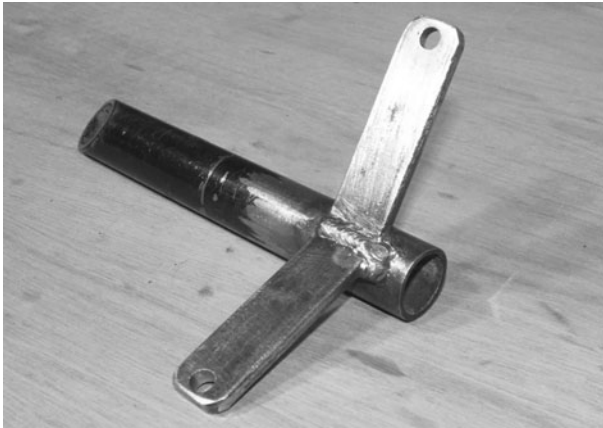
Figure 2-76 Fork mounting part completed
