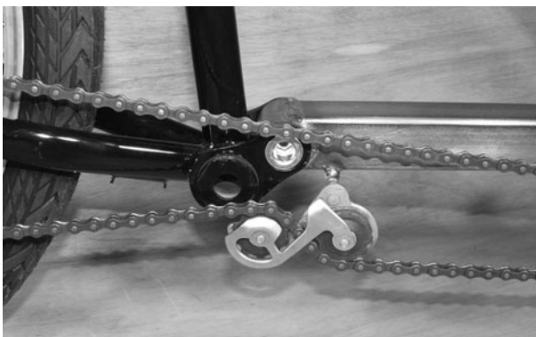
Figure 5-110 Installing the slack chain idler
