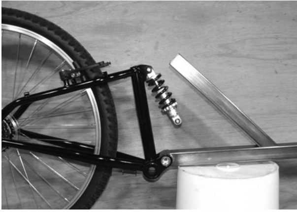
Figure 5-34 Looking for the optimal seat tube placement
