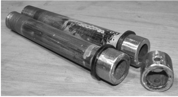
Figure 5-9 Fork crowns cut to 1 inch
