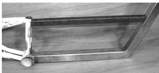
Figure 13-33 Installing the top tube
