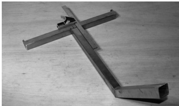
Figure 9-20 Joining the front and rear parts of the frame
