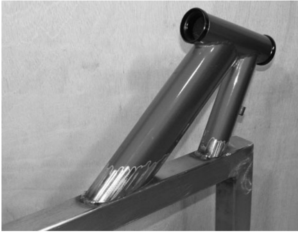
Figure 12-20 Head tube welded to the center frame
