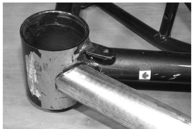
Figure 4-7 Grinding the tubing for a better weld
