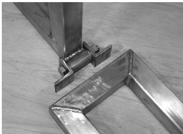
Figure 12-39 Connecting the swingarm
