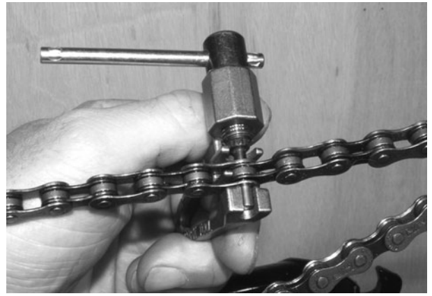
Figure 1-7 Removing the chain
