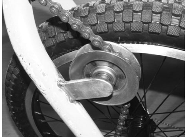
Figure 9-56 Pulley mounting tab tack welded in place
