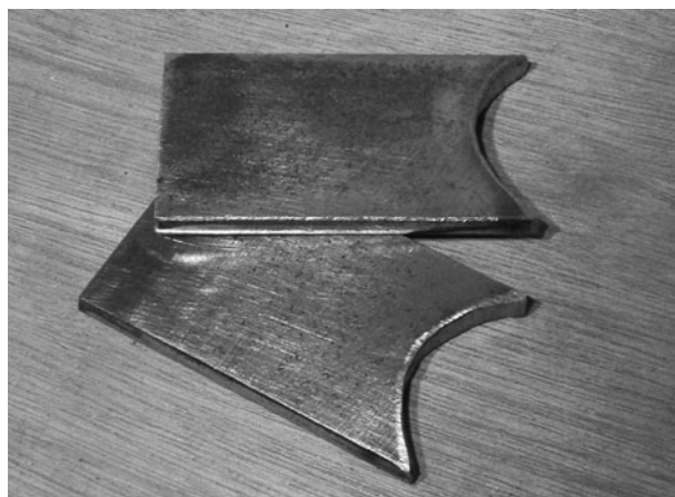
Figure 5-86 Shaping the bottom bracket plates
