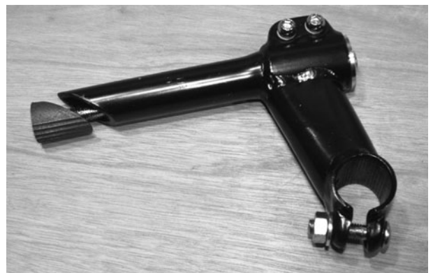
Figure 1-17 The wedge-shaped gooseneck clamp
