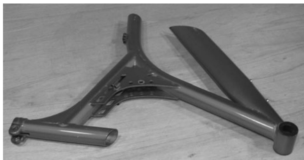
Figure 5-24 Remove the swing arm bearing tube
