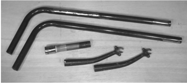
Figure 3-9 These parts will become the new forks
