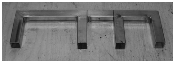
Figure 6-7 Welding the brake-side axle mount tube in place
