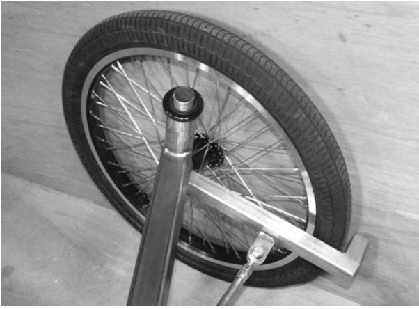
Figure 5-82 Ball joint and control arm closeup
