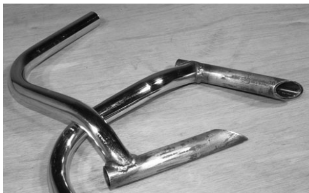
Figure 5-103 Handlebar halves completed
