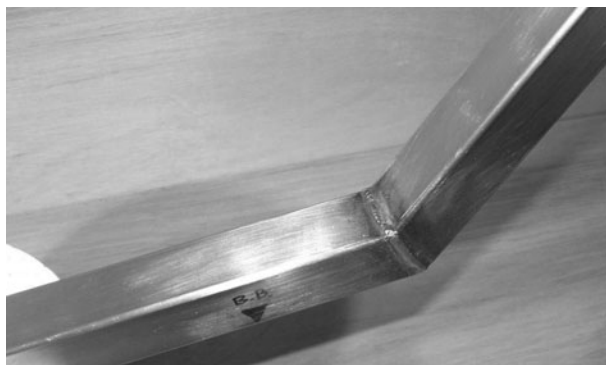
Figure 6-70 Front tube welding completed
