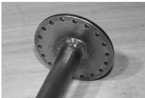
Figure 6-43 Inner joint fully welded
