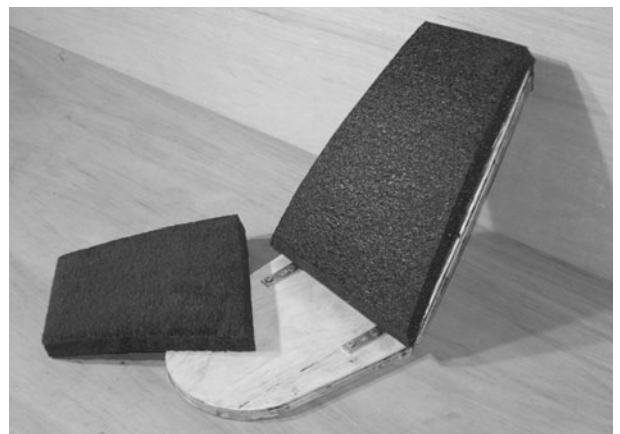
Figure 6-152 Gluing the foam to the wooden seat base
