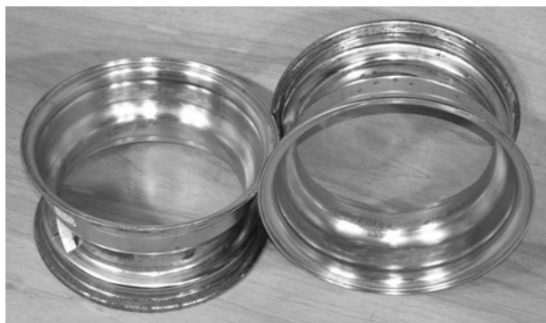
Figure 2-8 Repaired and sanded rims
