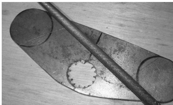
Figure 11-25 Hole ready for filing
