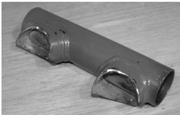
Figure 2-50 A head tube cut from an old frame
