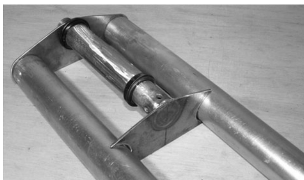
Figure 11-33 Setting up the fork set for welding
