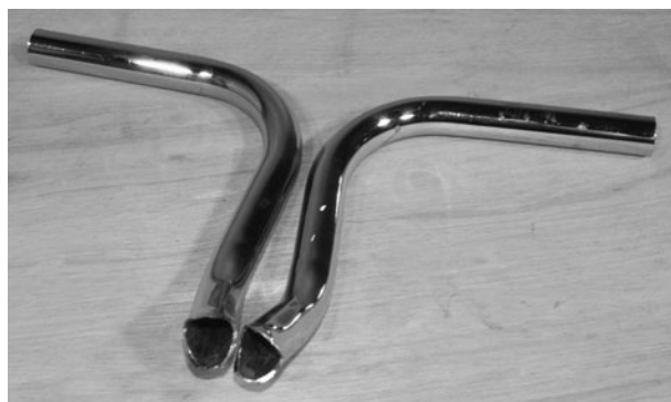
Figure 5-101 Cutting up the handlebars into two pieces
