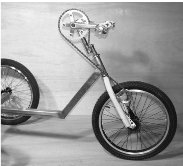
Figure 9-55 The chain will clear the fork legs
