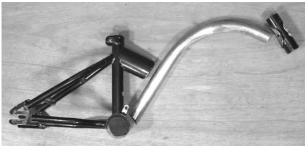
Figure 4-4 Using some bent conduit
