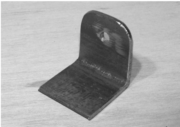
Figure 8-31 The top seat mount made of angle iron
