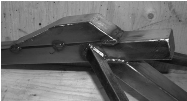
Figure 6-28 Only a few short welding beads are needed
