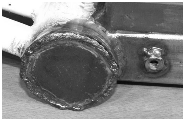
Figure 13-62 Welding the caps in place
