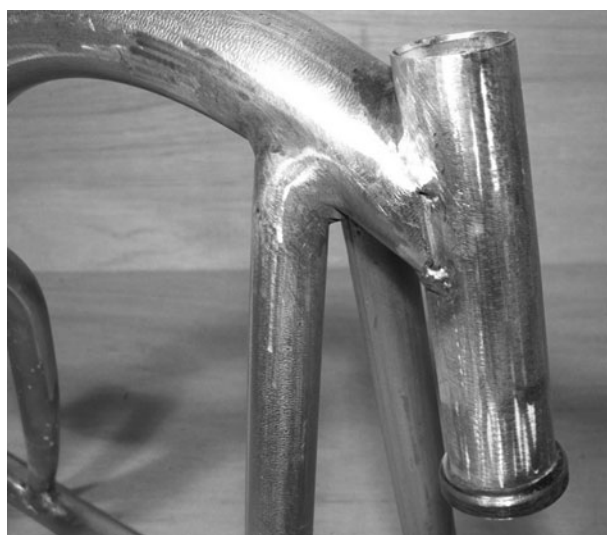
Figure 11-38 Weld the sides of the joint last
