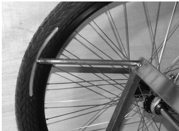
Figure 6-138 Mounting the guard arms to the frame
