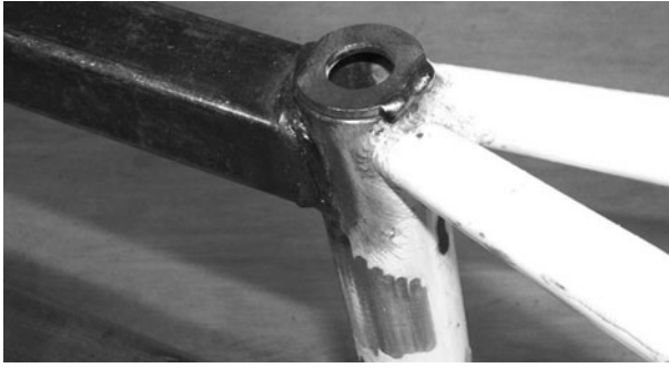
Figure 13-37 Capping the top of the seat tube
