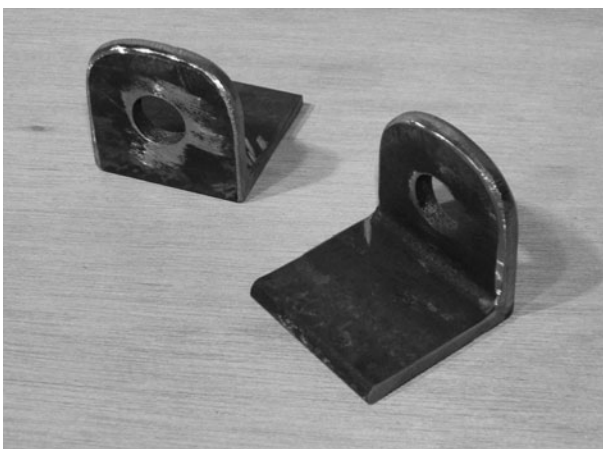
Figure 8-15 Rear caster mounts are cut, drilled, and rounded for safety
