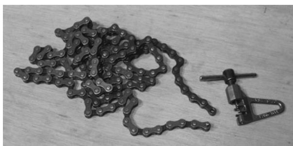
Figure 9-65 Creating the correct length chain
