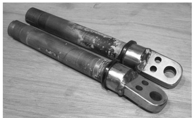
Figure 5-22 Axle mounting tabs fully welded
