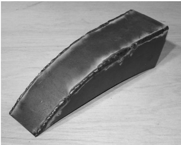
Figure 8-38 Welding the fender parts together
