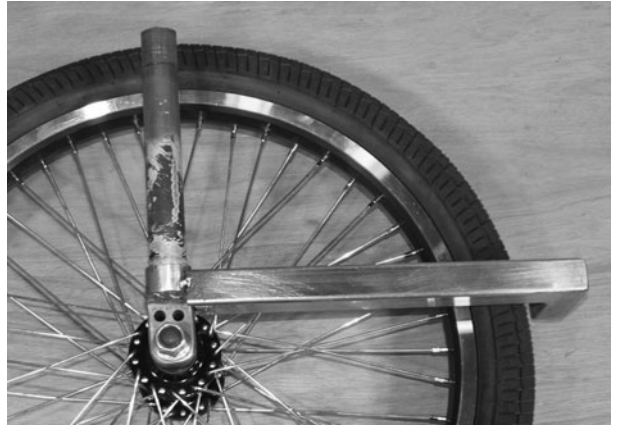
Figure 5-69 Installing the brake support arms
