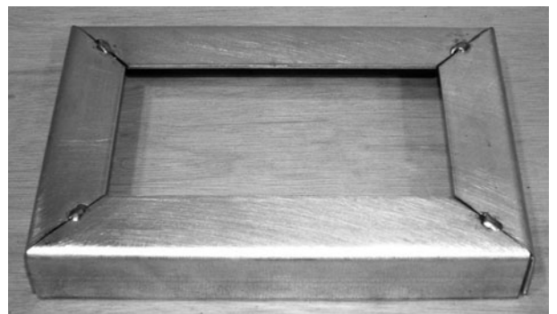
Figure 12-10 Tack welded battery pack base
