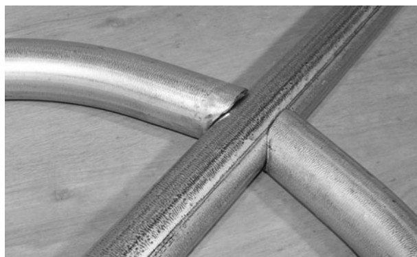
Figure 2-37 Grinding out tubes for a better weld
