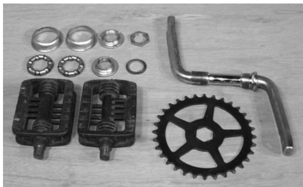
Figure 7-3 Cleaning up the crank set hardware
