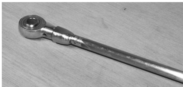
Figure 6-111 Mounting the ball joints to the connecting rod
