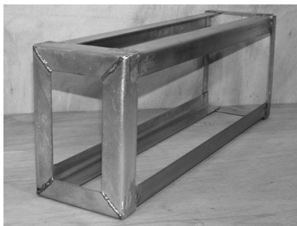
Figure 12-13 Battery pack welding completed
