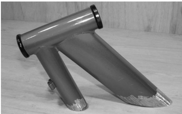
Figure 12-4 The front of the frame has been cut
