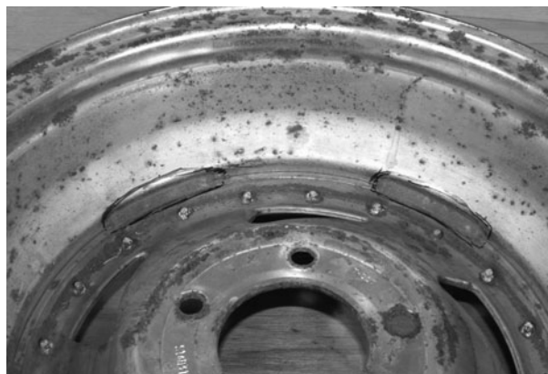
Figure 2-2 The center of the rim is welded in place
