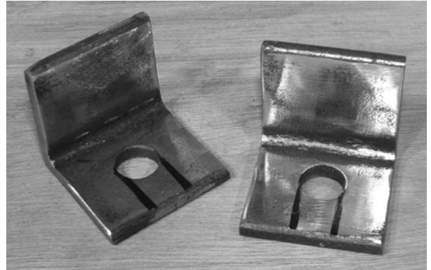
Figure 12-31 Drilling the axle holes
