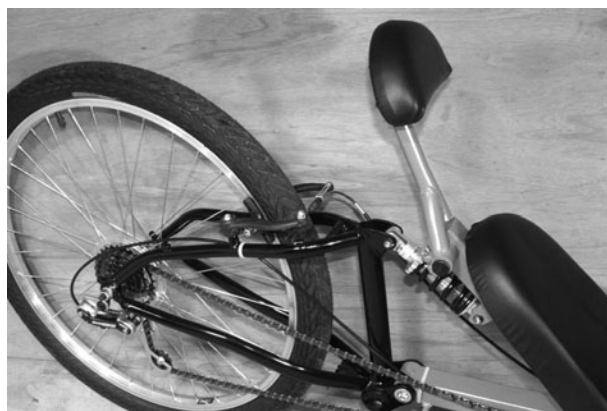
Figure 5-127 Setting up the rear brake
