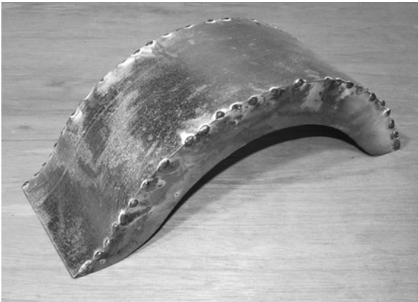
Figure 11-77 Tack welded fender
