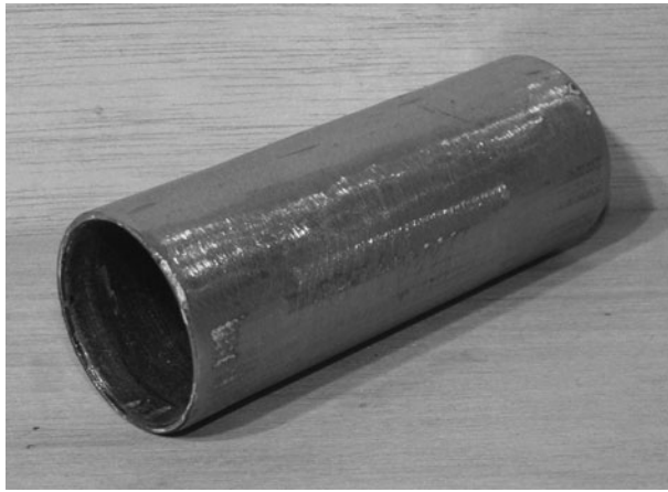
Figure 6-66 Grind the head tube clean
