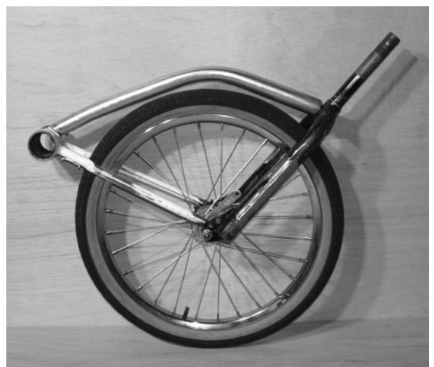
Figure 8-11 Test fitting the front wheel in place to check clearance
