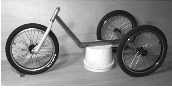
Figure 9-30 Setting up the head tube angle
