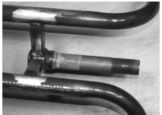
Figure 3-13 Installing the fork stem
