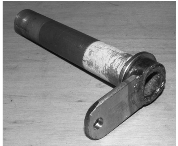
Figure 6-82 Weld the control arm to the fork stem
