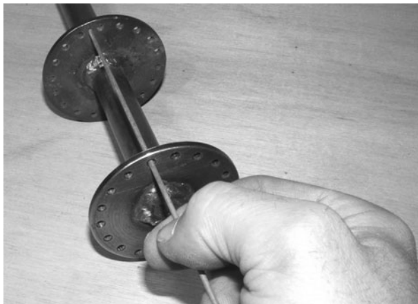
Figure 6-45 Holes in opposing flanges are offset by each other
