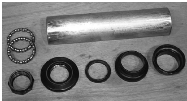
Figure 2-58 Checking the fork hardware
