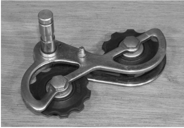
Figure 5-109 Removing most of the derailleur parts
