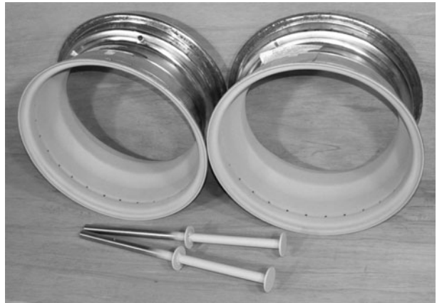
Figure 2-22 Hub axles and rims getting primer
