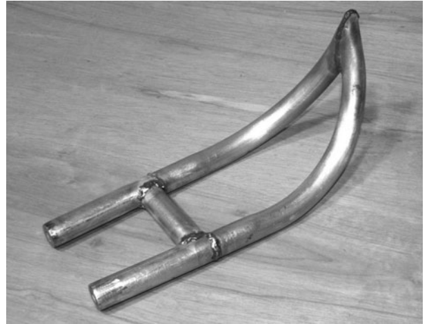
Figure 12-53 A motocross-style seat mount
