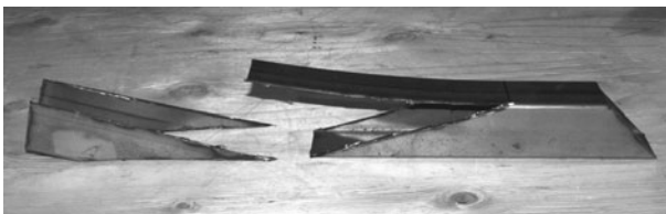
Figure 6-24 A neat cutting trick to reduce welding a bit
