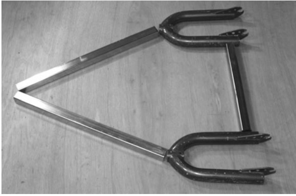
Figure 14-6 Laying out the basic frame
