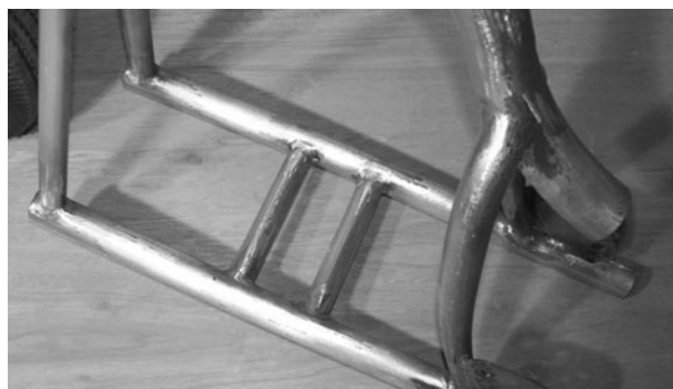
Figure 11-56 Motor mounting tubes welded in place
