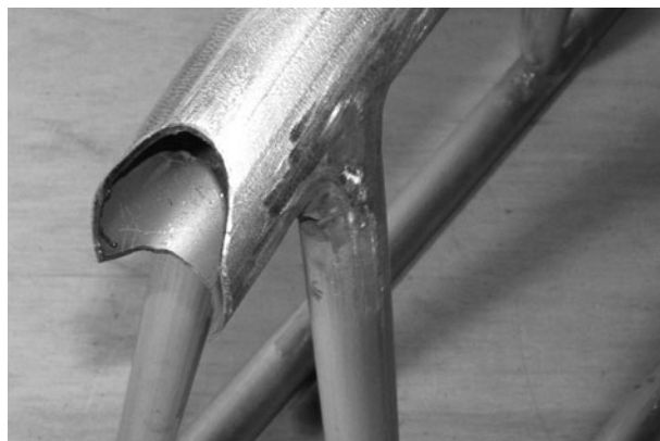
Figure 11-35 Head tube joint ground
