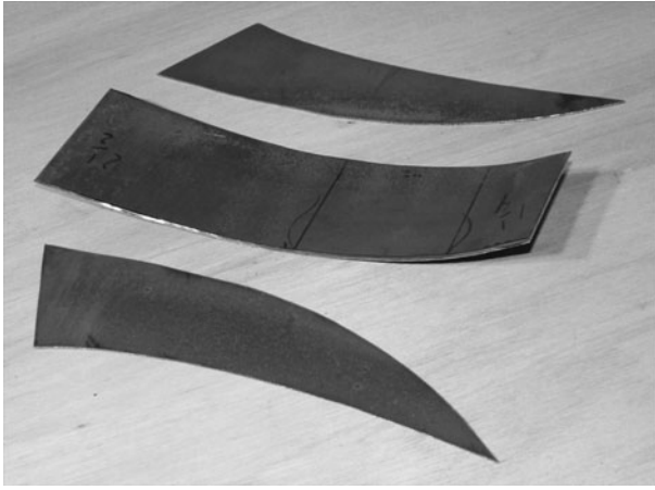
Figure 8-37 Making the fender to stop wheel rubbing
