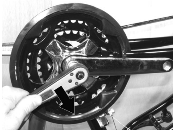
Figure 1-12 Removing the crank axle bolt
