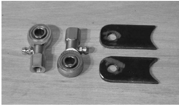
Figure 6-81 The two ball joints and the control arms
