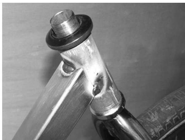
Figure 6-73 Tack welding the head tube a little at a time
