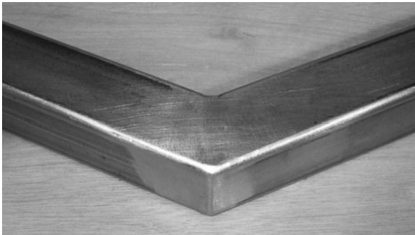
Figure 5-42 Front arm tube joint cleaned up
