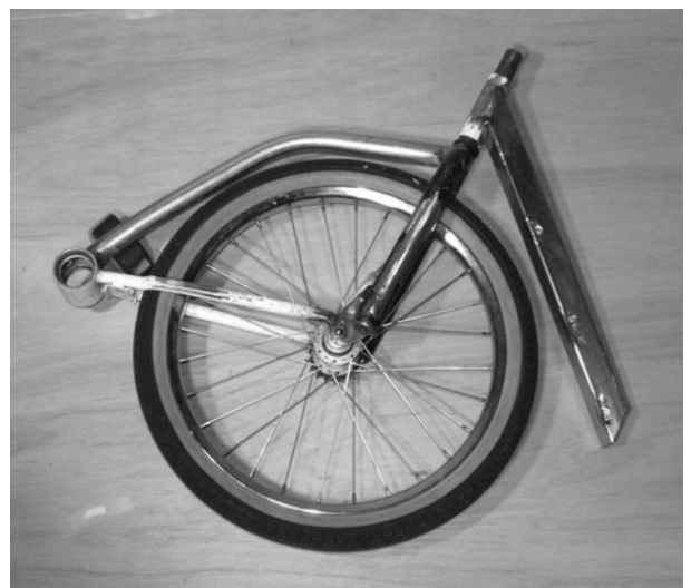
Figure 8-22 Front tube length is based on ground clearance and fork angle
