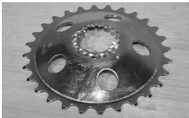
Figure 2-80 Making a hole in the sprocket
