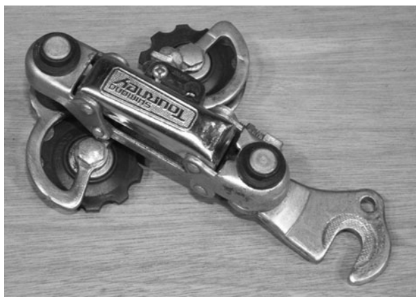
Figure 5-108 Making a chain slack pickup idler
