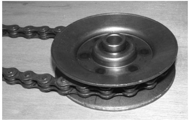
Figure 9-52 The chain should fit in the pulley groove
