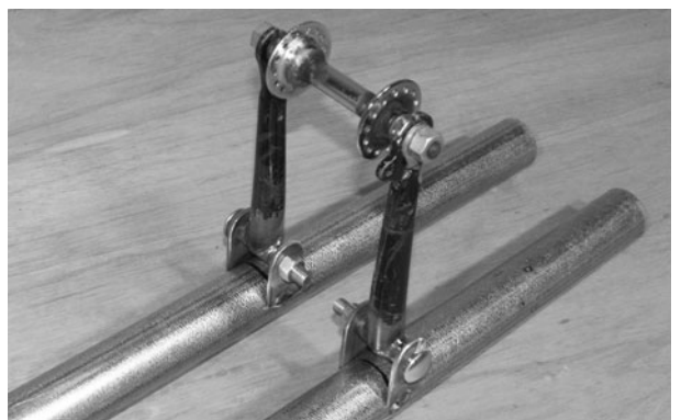
Figure 2-62 Installing the suspension parts
