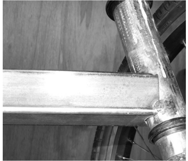
Figure 5-58 Two tack welds secure the head tube
