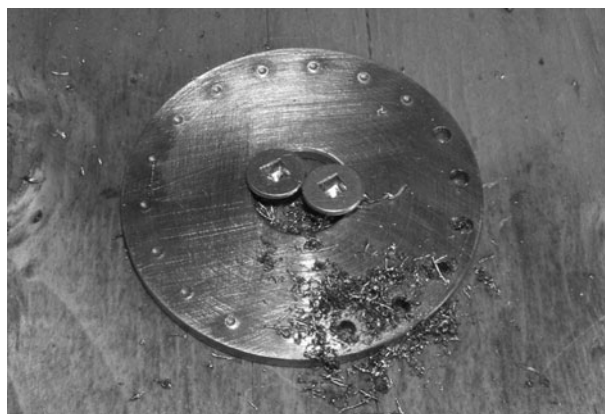
Figure 6-32 Drilling the spoke holes
