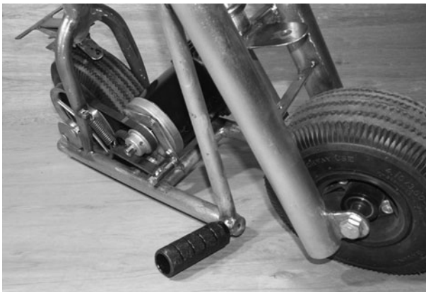
Figure 11-85 Foot pegs are installed to allow the bike to lean in turns
