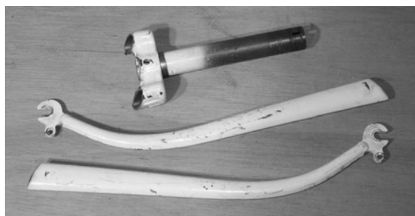
Figure 6-133 Cut the fork legs at the crown
