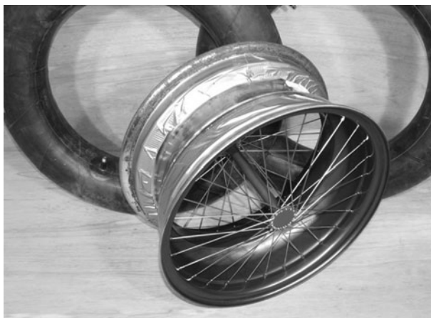
Figure 2-32 Cover the spoke nipples with duct tape
