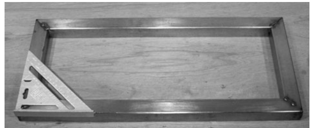
Figure 12-16 Squaring up the center frame
