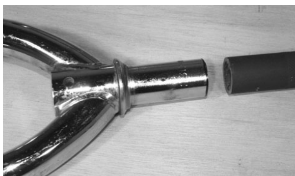
Figure 10-6 Extending the fork stem
