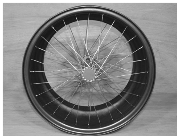
Figure 2-27 All crossing spokes are now installed on one side
