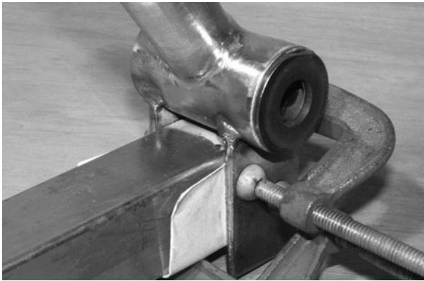
Figure 5-89 Tack welding the plates to the bottom bracket
