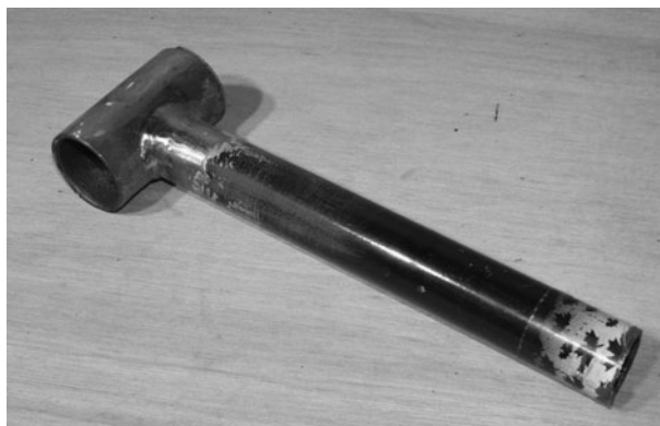
Figure 6-93 Bottom bracket cut and ground clean
