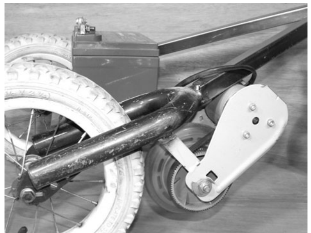
Figure 14-13 Installing the motor
