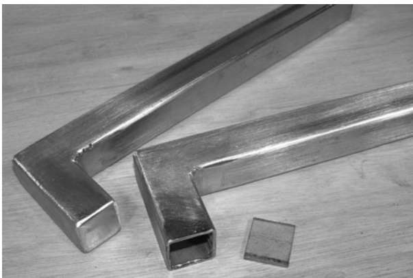
Figure 5-68 Capping the open ends of the tube
