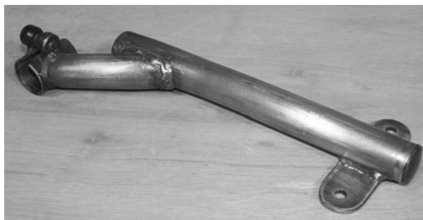
Figure 5-106 Backrest mounting tabs
