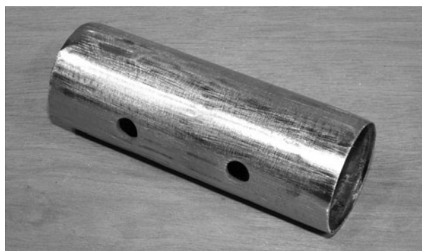
Figure 13-8 Cleaning up the head tube
