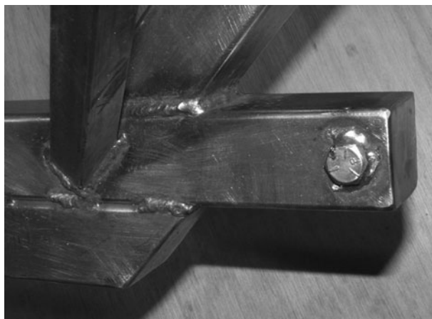
Figure 6-118 Securing the idler pulley bolt
