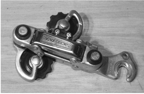
Figure 9-58 An old road bike rear derailleur
