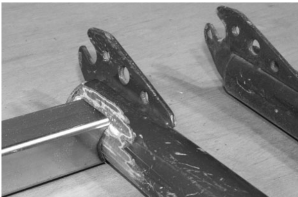
Figure 14-7 Joining the two rear forks together
