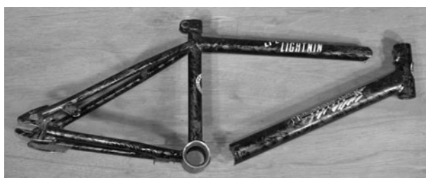
Figure 7-4 The first cut made to both matching frames
