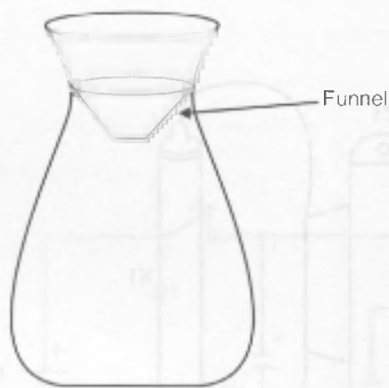
Figure 3.11.7 Preventing the insects from escaping from the trap
