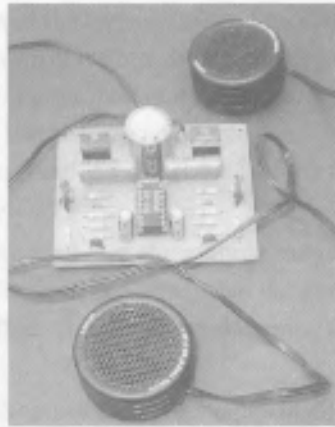
Figure 3.7.7 Panic generator mounted on a PCB
