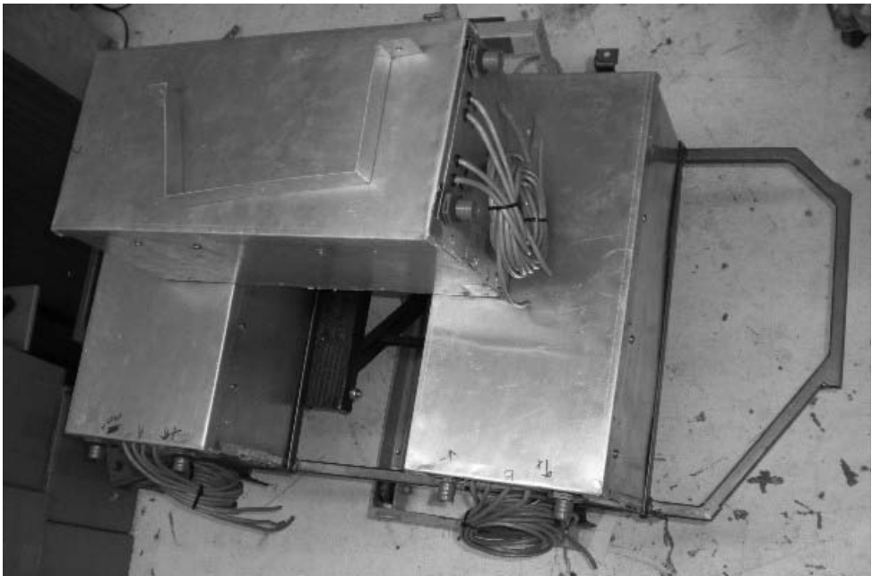
FIGURE 10-9 Electric motor mount from EVP orsche.com.
