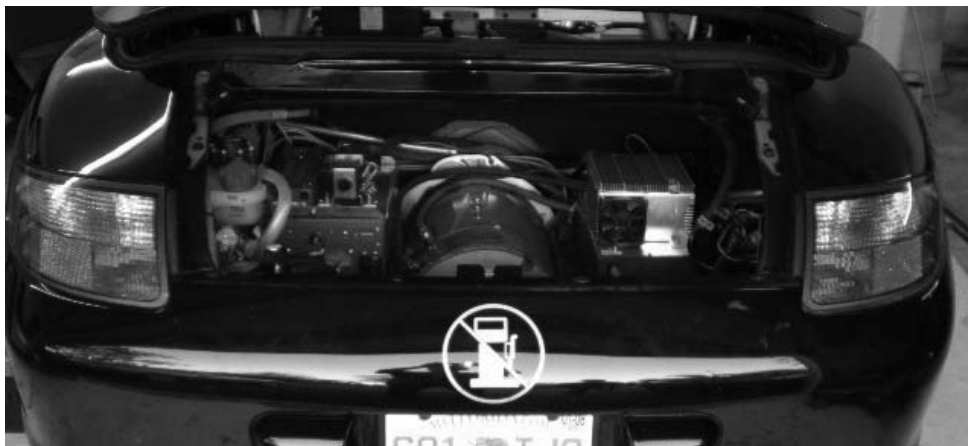
FIGURE 10-19 Porsche electric motor power cabling in the trunk.
