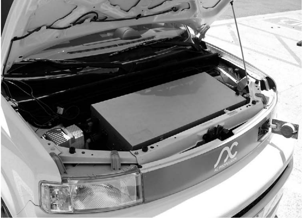
FIGURE 7-9 AC Propulsion 120kW power electronics drivetrain in the eBox.
