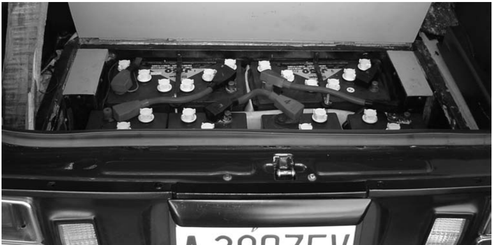
FIGURE 4-11 Joe Porcelli and Dave Kimmins of Operation Z's Nissan 280Z rear battery compartment.
