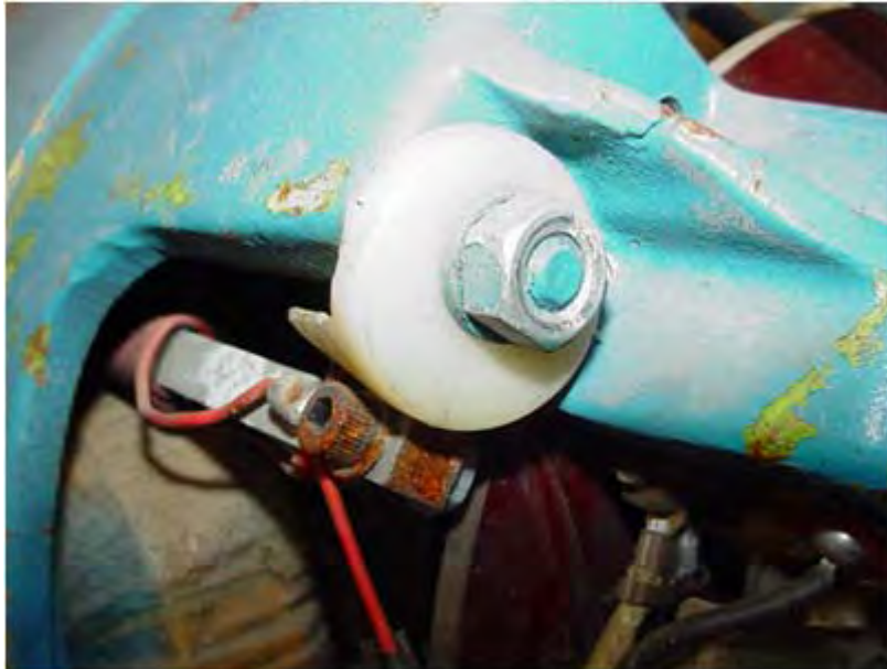
Added Magnetic Probe Next to Stator Winding Assumed Used for Positional Feedback
