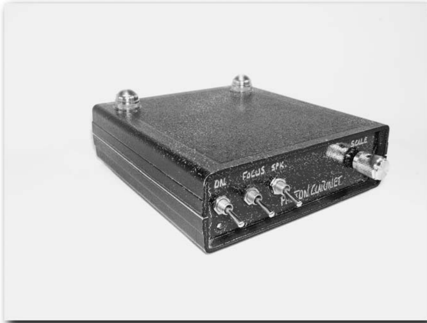
FIGURE 11-8: Photon clarinet in plastic project box
