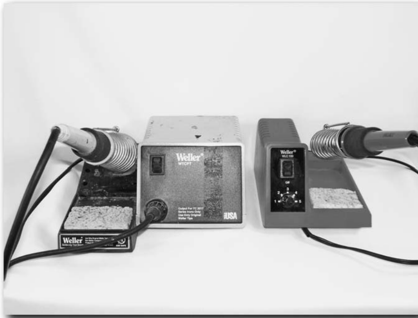
FIGURE 5-1: Weller soldering stations: the WTCPT on the left, the WLC100 on the right
