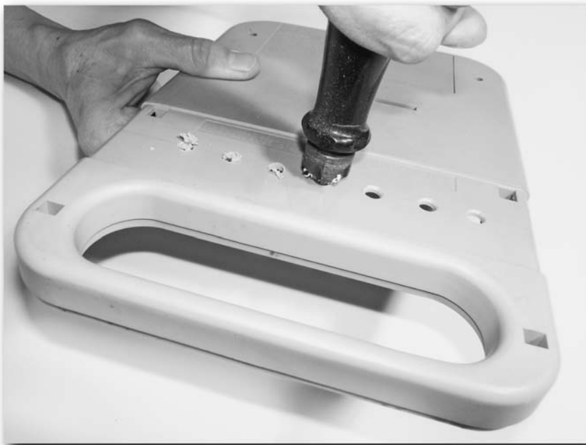
FIGURE 10-9: Use a de-burrer to smooth hole edges.
