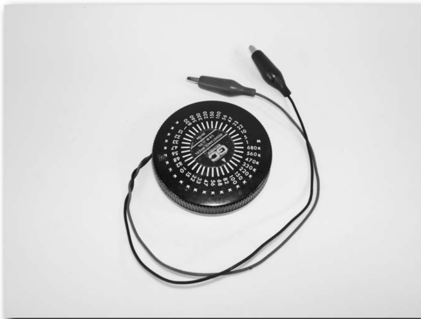
FIGURE 6-11: A resistor substitution wheel
