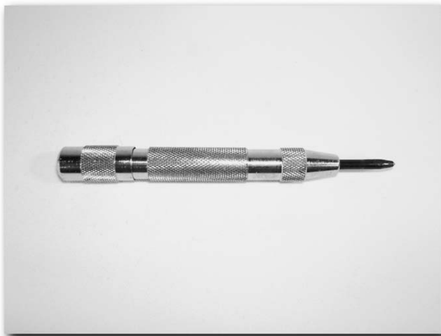
FIGURE 10-6: Use a center punch for locating holes to be drilled in metal.
