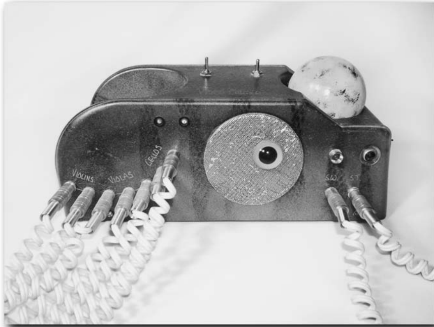
FIGURE 11-14: The Video Octavox in unusual telephone handset case
