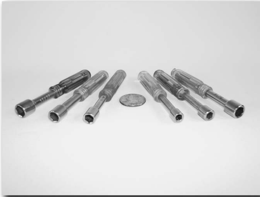
FIGURE 5-7: Socket drivers with hollow shafts
