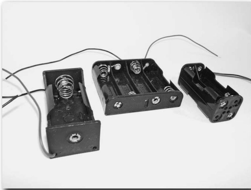
FIGURE 6-27: Assorted battery holders
