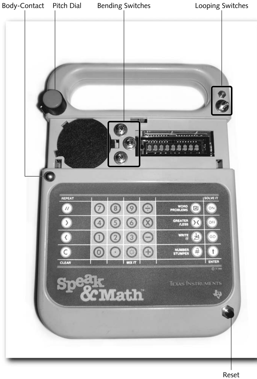
FIGURE 17-1: Speak & Math in standard Incantor configuration
