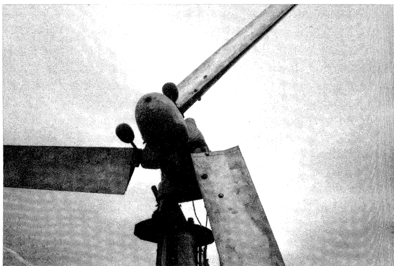
Dunlite centrifugal pitch control mechanism.
