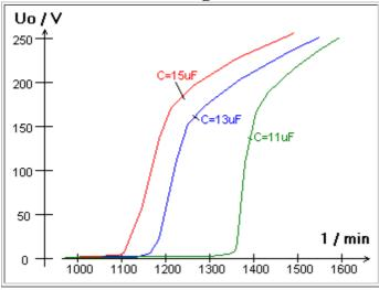
The idle or loadless voltage voltage of the generator with several capacitive values. The voltage rises when the capacitance increases.
