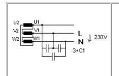
If motor/generator is connected as a triangle there is a monophase voltage available between two phases. The nominal voltages of the motor must be 220/380V too (nowadays 230/400V).
