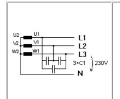
380/220V 3-phase squirrel motor, power 1,5 kW, nominal speed 1415 rpm.
