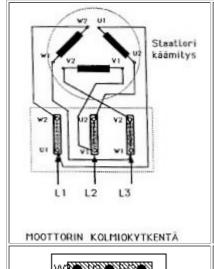
The connection box of the squirrel motor. The triangle connection seen here.
