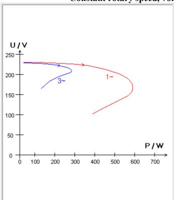
Capacitors 3 pcs 11uF each. Constant speed 1550 rpm.
