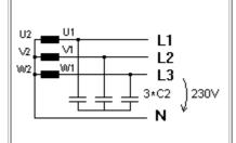
If the capacitors are connected as a star then their capacitances must to be triple as above or 3 pcs 33-45 uF each. Sustain voltage according the phase voltage 220V plus rich reserve. Maybe 300VAC (420VDC).
