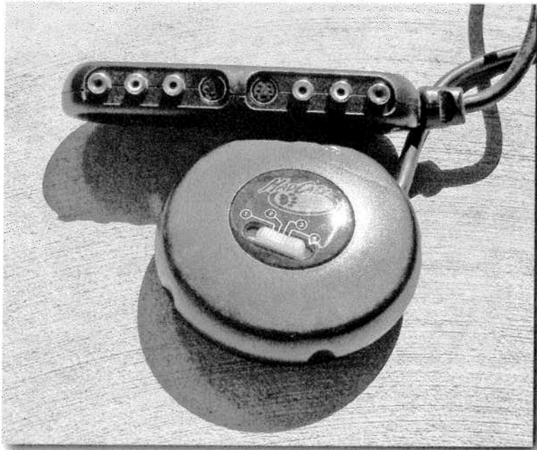
FIGURE 7-15: An analog video-analog switch you can pick up from practically any store.
