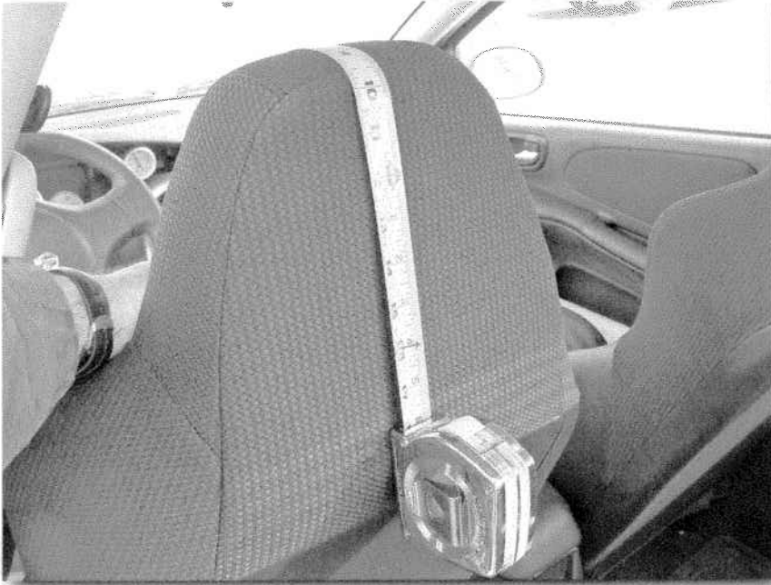
FIGURE 7-17: Measuring from the front to the back of the headrest portion of the seat.
