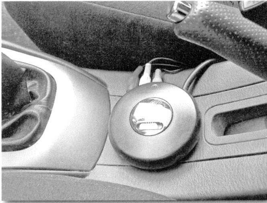
FIGURE 10-6: Installed A/V switch.
