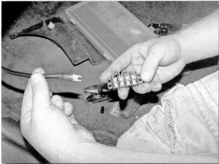
FIGURE 3-26: The power cable with attached ring connector and the bridged barrier terminal strip it connects to.
