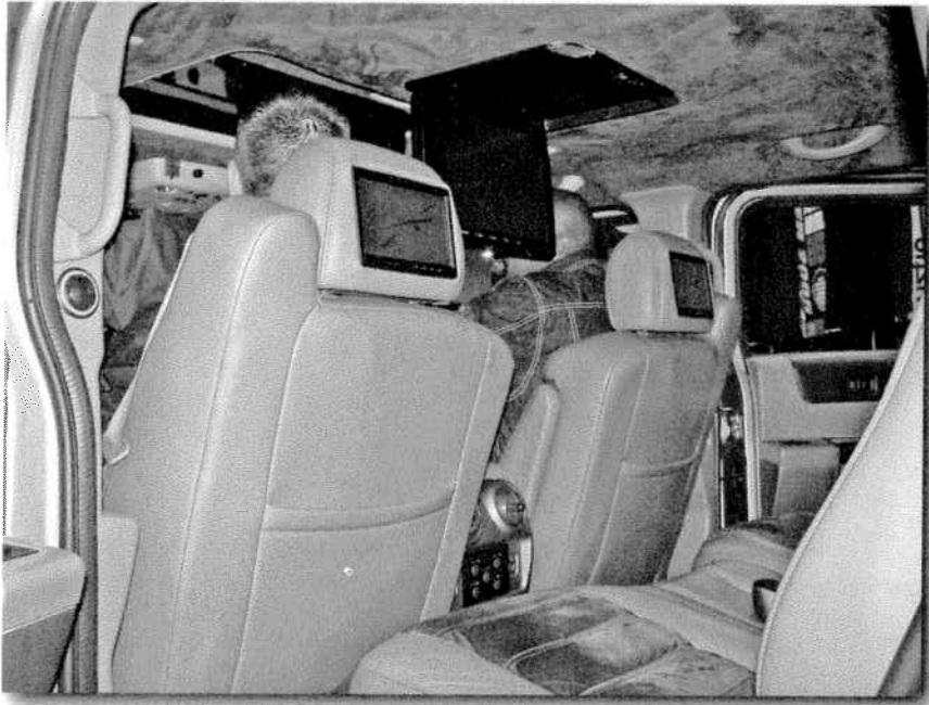
FIGURE 10-7: Seat-back displays let passengers play games or watch movies while you use your GPS in the front.
