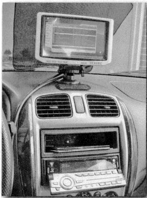
FIGURE 1-2: The display is mountable and can be removed just by turning a knob and is also small enough to fit in the glove compartment.
