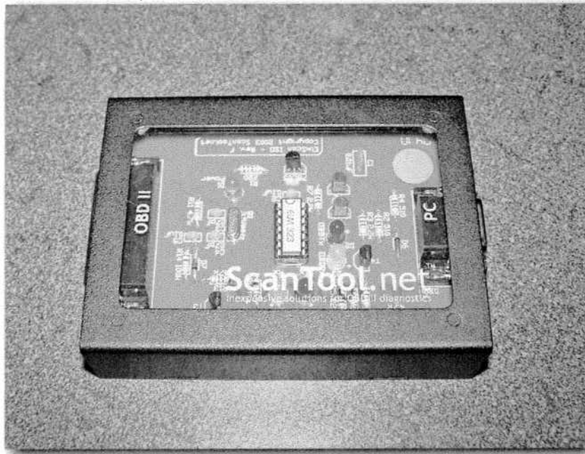
FIGURE 21-2: My jerry-rigged reader moved to the ScanTool enclosure.
