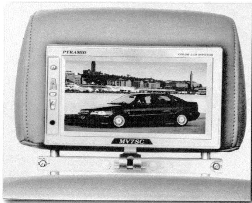
FIGURE 7-11: A display attached to the support bars on a headrest.
