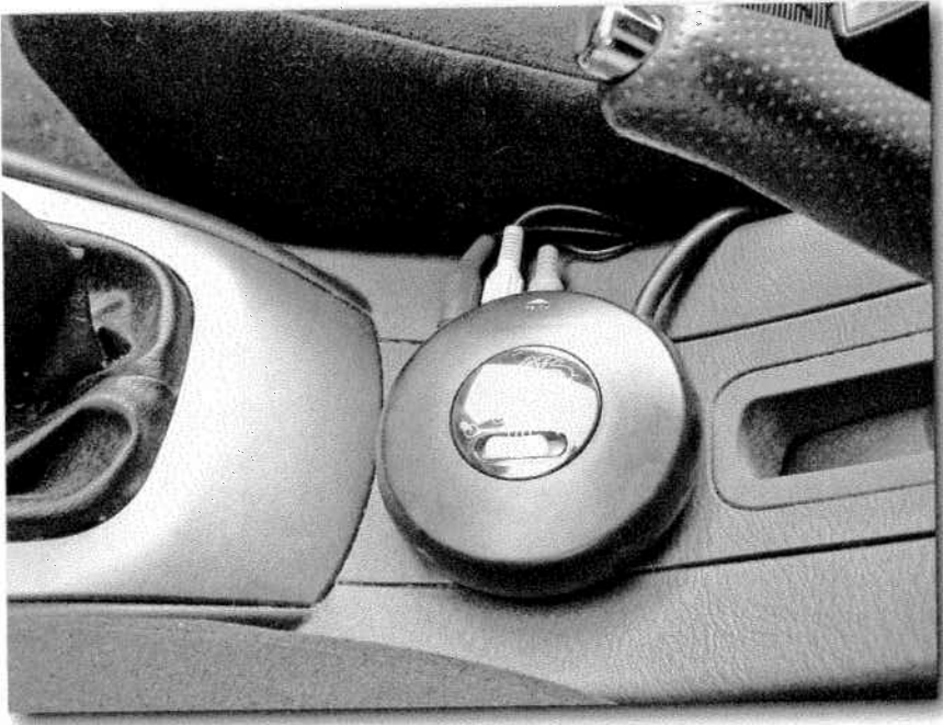
FIGURE 23-4: The installed A/V switch.
