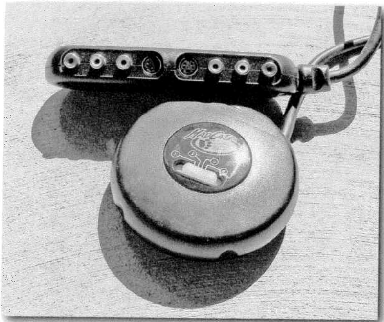
FIGURE 16-5: An A/V switcher.
