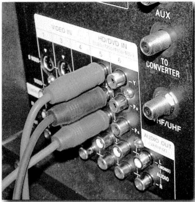
FIGURE 7-3: A set of component video cables (Y, Pr, and Pb), and the connectors they plug into.
