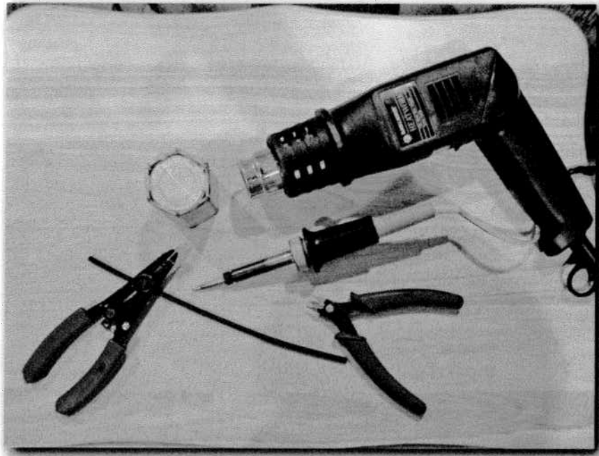
FIGURE 3-5: Tools used include a soldering iron, needle-nose pliers, wire cutter, shrink tubing, and soldering wire.
