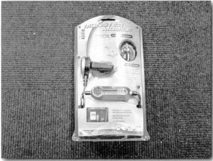
FIGURE 9-5: An FM radio audio transmitter can be quite convenient if you don't want to spend money on a new head unit.
