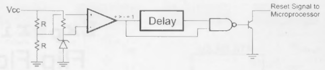
Figure 12-16 Possible microprocessor reset circuit
