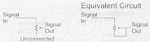
Figure 3-31 Wiring a potentiometer as a variable resistor
