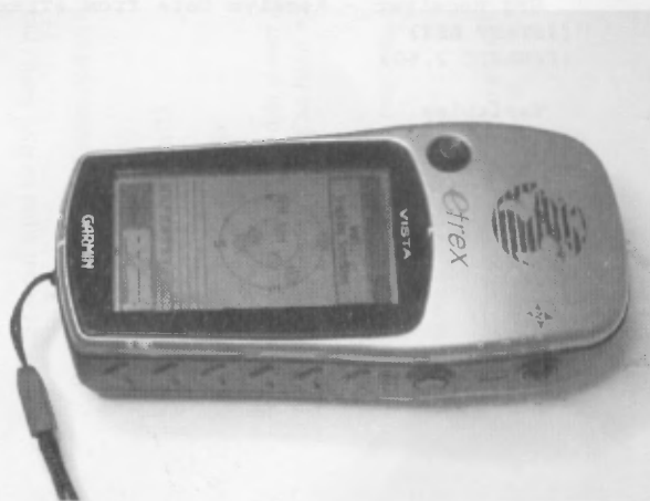
Figure 17-17 The Garmin eTrex provides position and heading information via an NMEA interface as well as a moving map display.
