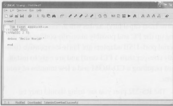
Figure 13-7 Screen shot of the BASIC Stamp Windows Editor with the first program entered in
