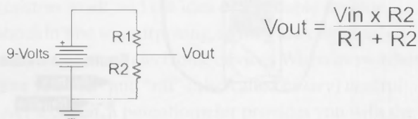
Figure 3-30 Breaking the single resistor in a potentiometer into two to create a voltage divider
