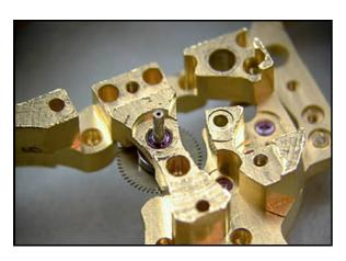
On the dial side of the movement (**right**) we find a conventional cannon pinion (1) to carry the minute hand hand, as well as a minute wheel (2) to drive the hour hand. Even the hand-setting mechanism employs an intermediate wheel (3) that could be lifted from the most traditional of mechanical movements.
