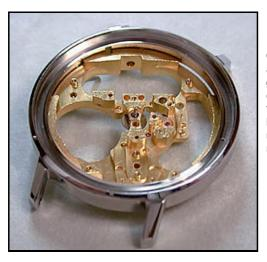
On first examination, one of the most startling aspects of the Accutron is how much traditional, high grade watchmaking is involved in its design and execution. It uses an extremely well-made, traditional, machined brass ebauche (left) with a highly jeweled gear train. Most of the gear train uses conical pivots with pierced and cap jewels, and nearly half the gear train is shock protected.
