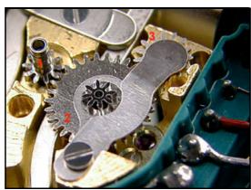
The gear train of the Accutron resembles that of a high-grade mechanical movement (**right**). We might even imagine that we were observing a center wheel (1), third wheel (2), fourth wheel (3), escape wheel (4), and . . . well, it's not a balance wheel, its the *drive wheel* (5). More about that drive wheel in a moment.
