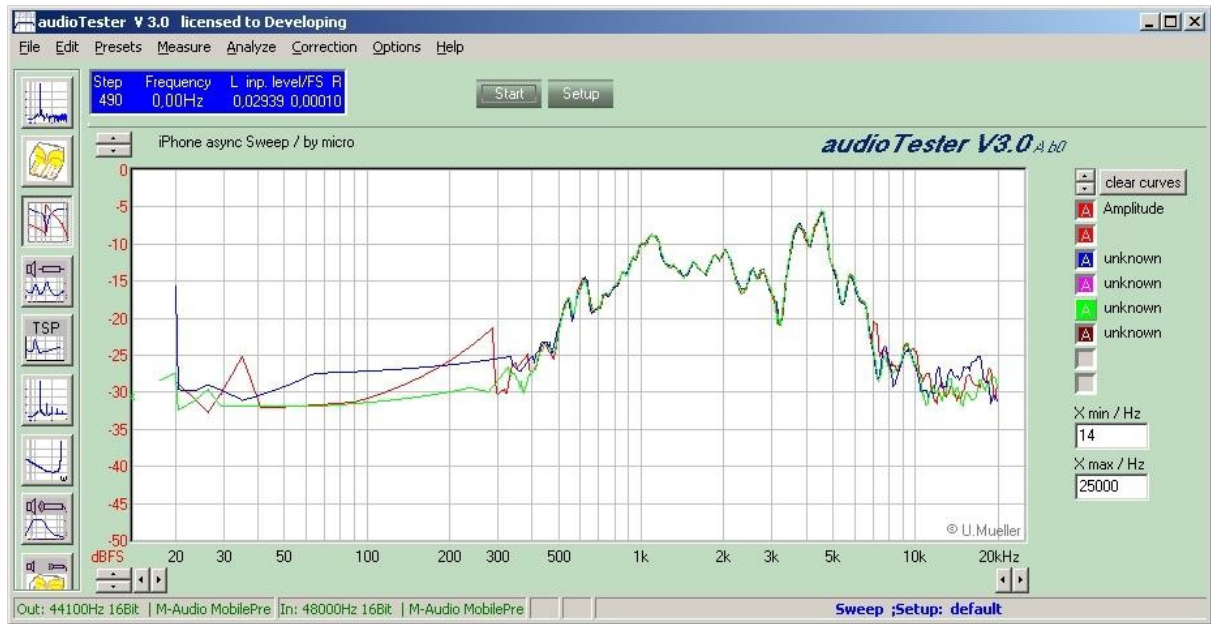
Measure microphone 20mm over iPhone Speaker Measurement repeat 3 times (red,blue,green), values below 300Hz not analysable
